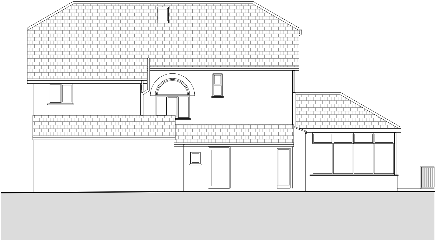
EXISTING REAR ELEVATION 1:100 @ A3
