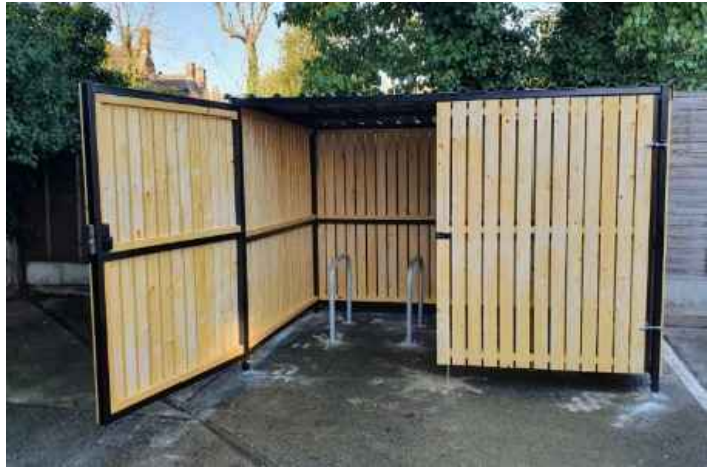
TRINITY TIMBER WOODEN BIKE SHELTER FOR SECURE SAFE STORAGE FOR 6 CYCLES. MADE FROM 50x50x3mm MILD STEEL BOX FRAME, WITH ROUGH SAWN TIMBER CLADDING, AND DOUBLE DOOR OF TIMBER CLADDING WITH 3 HINGE ANTI-LIFT DOORS. BEING 2350mm DEPP AND 2650mm WIDE, AND A HEIGHT OF 2150mm HIGH. WITH 3 NO SHEFFIELD TOAST RACK, SECURE DOWN TO CONCRETE BASE.
