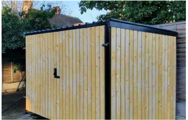
TRINITY TIMBER WOODEN BIKE SHELTER FOR SECURE SAFE STORAGE FOR 6 CYCLES. MADE FROM 50x50x3mm MILD STEEL BOX FRAME, WITH ROUGH SAWN TIMBER CLADDING, AND DOUBLE DOOR OF TIMBER CLADDING WITH 3 HINGE ANTI-LIFT DOORS. BEING 2350mm DEPP AND 2650mm WIDE, AND A HEIGHT OF 2150mm HIGH. WITH 3 NO SHEFFIELD TOAST RACK, SECURE DOWN TO CONCRETE BASE.
