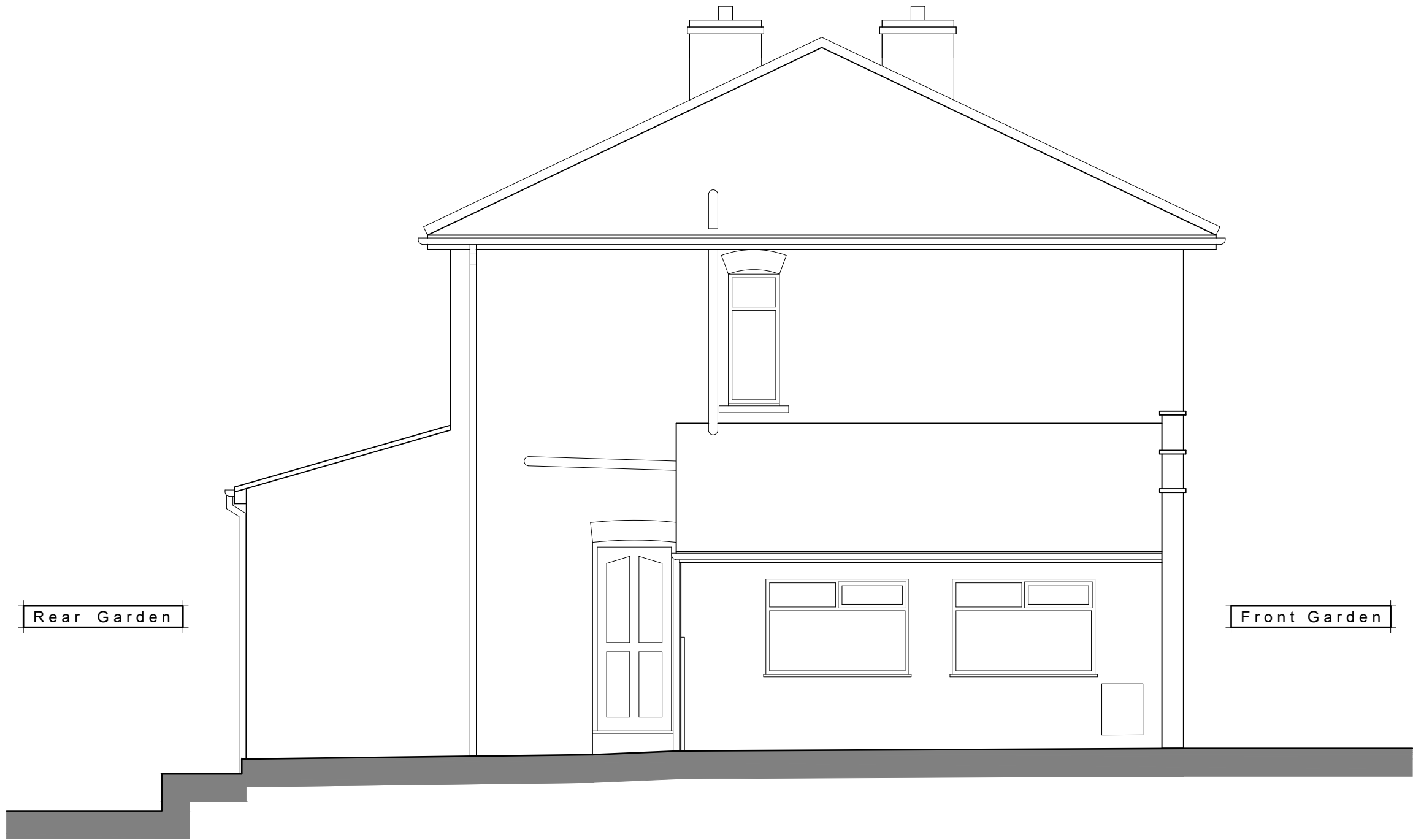
Existing Side Elevation 1:50
