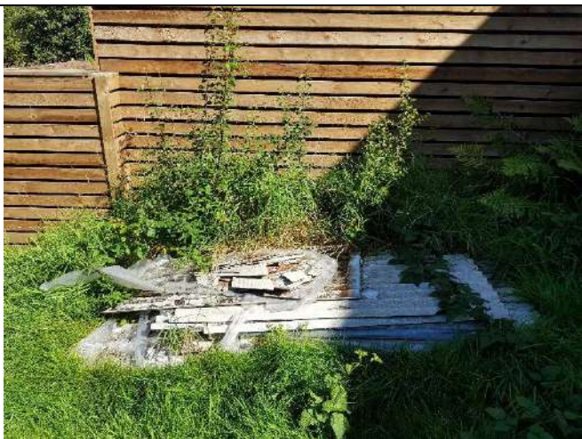
P13: Suspected asbestos cement sheeting present to the rear of 45 Ajax Drive adjacent to the north-eastern site boundary
