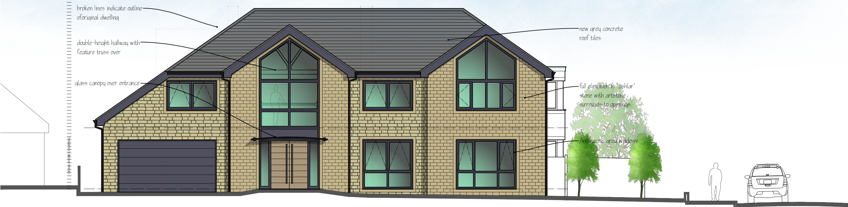
ELEVATION ALONG WINDRUSH AVENUE
