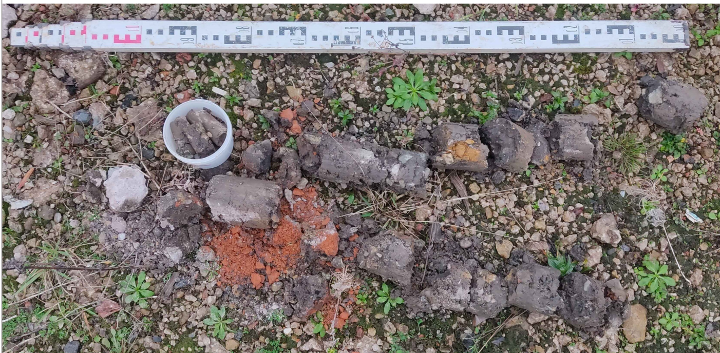
Image 1. DS02: Viewed right to left, top to bottom 0.00m - 1.20m bgl. 1.20m - 1.50m bgl.
