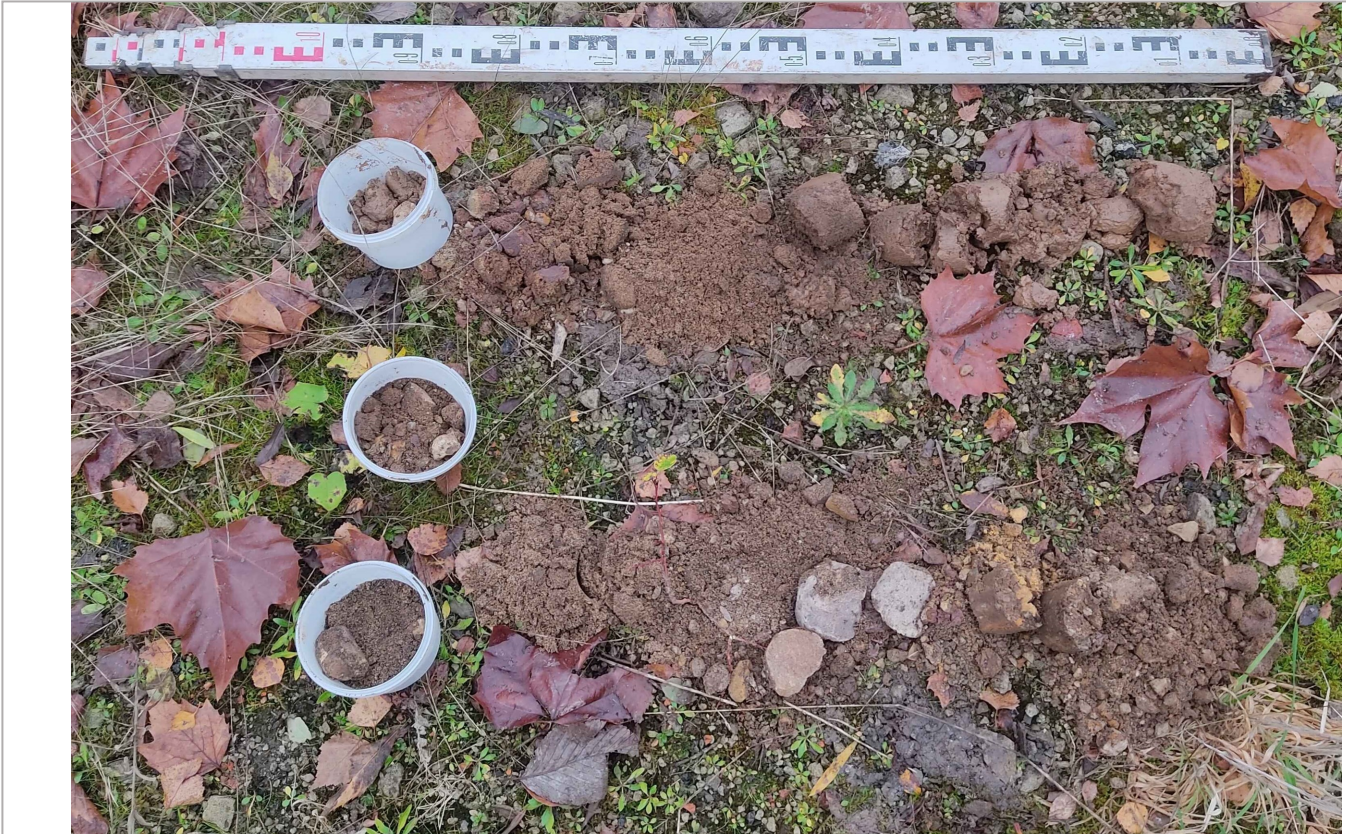
Image 1. DS05: Viewed right to left, top to bottom. 1.20m - 2.00m bgl. 2.00m - 3.00m bgl.
