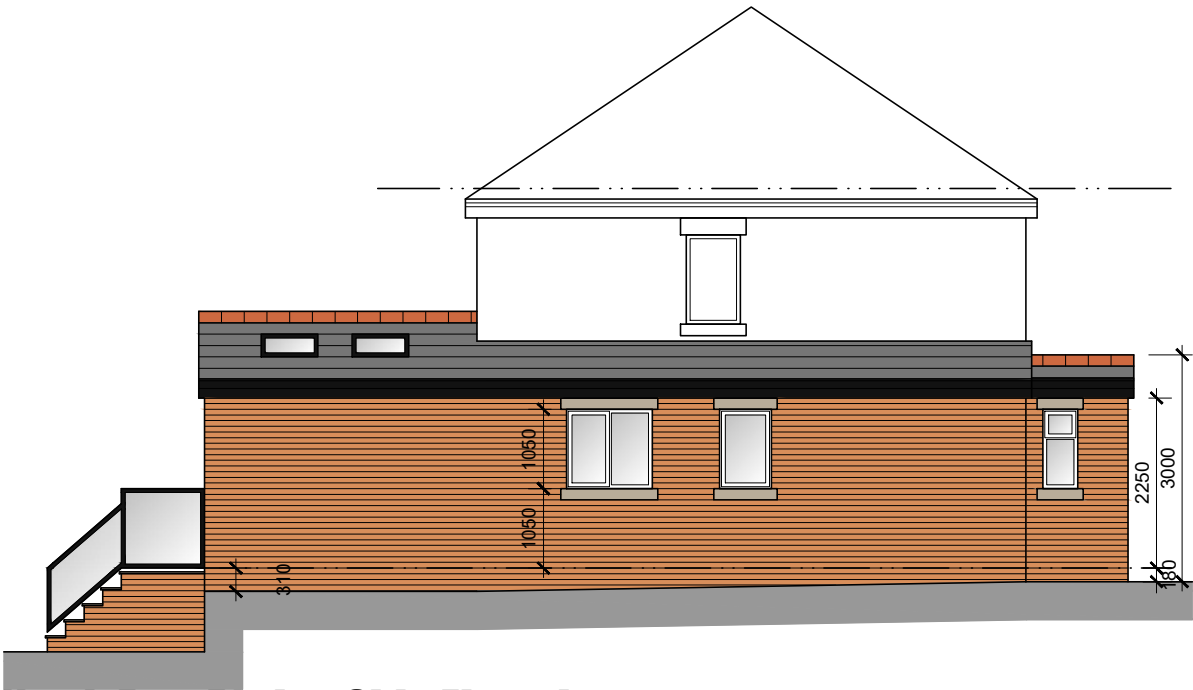
North East Facing Side Elevation
