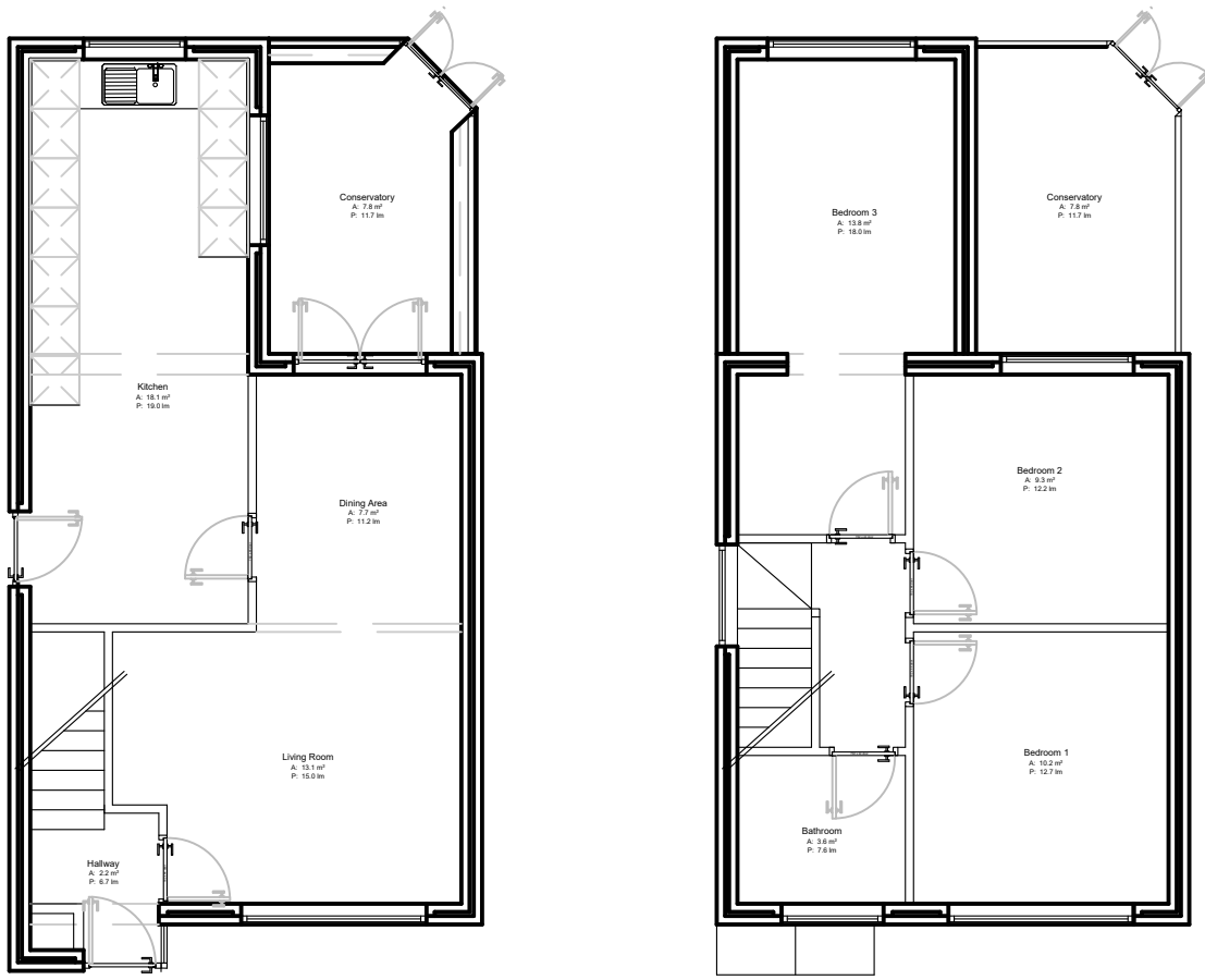
Existing Gnd & 1st Floor Plans @ 1:100
