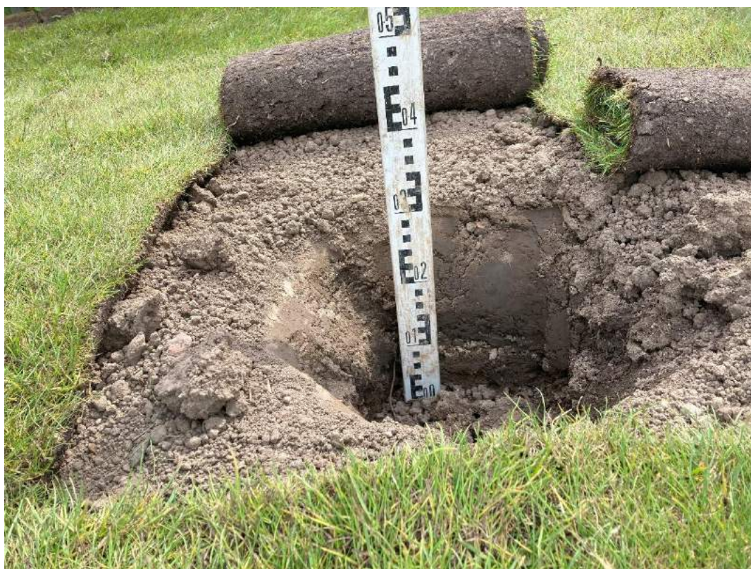
Plate 18 – HP04 GL to 0.3m bgl with 0.15m of topsoil.
