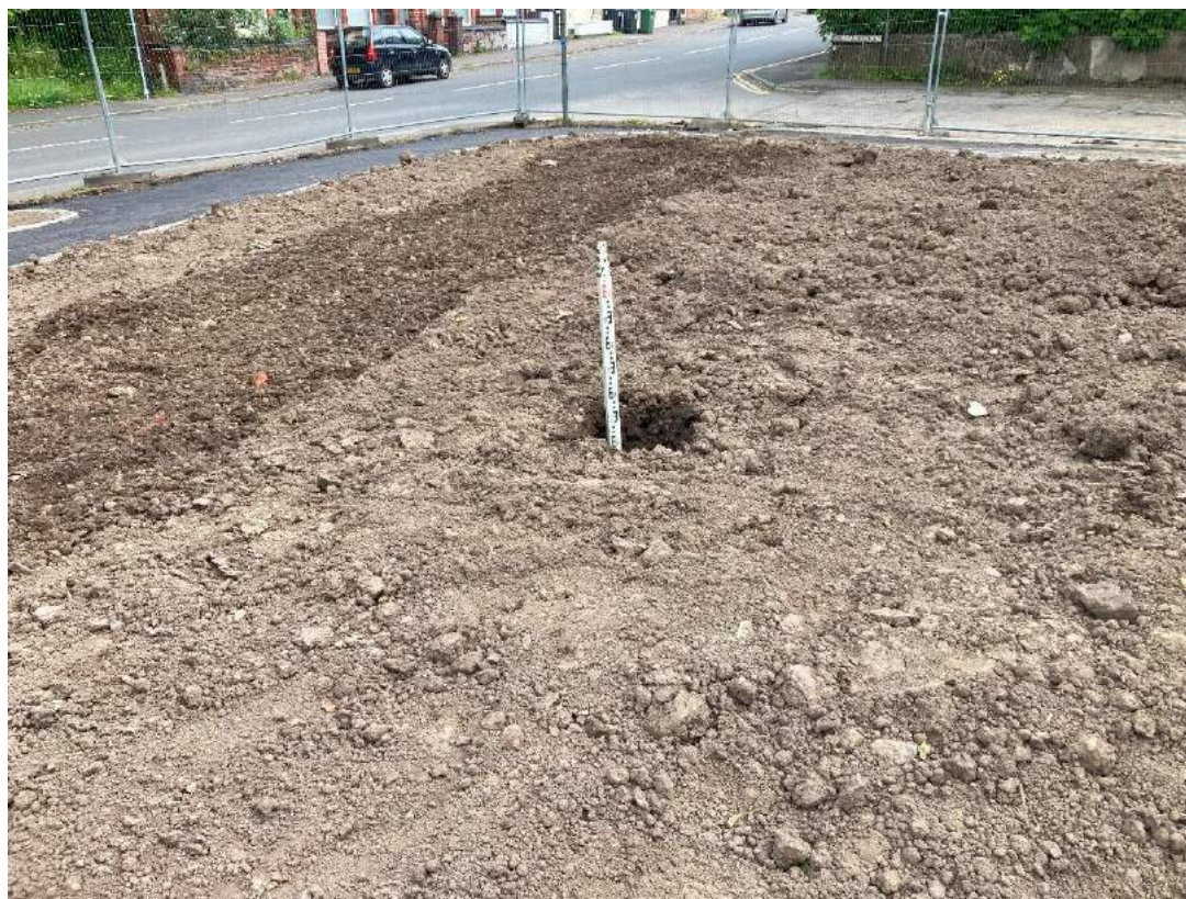
Plate 20 – HP05 GL to 0.60mbgl and arisings, with 0.20m of topsoil.
