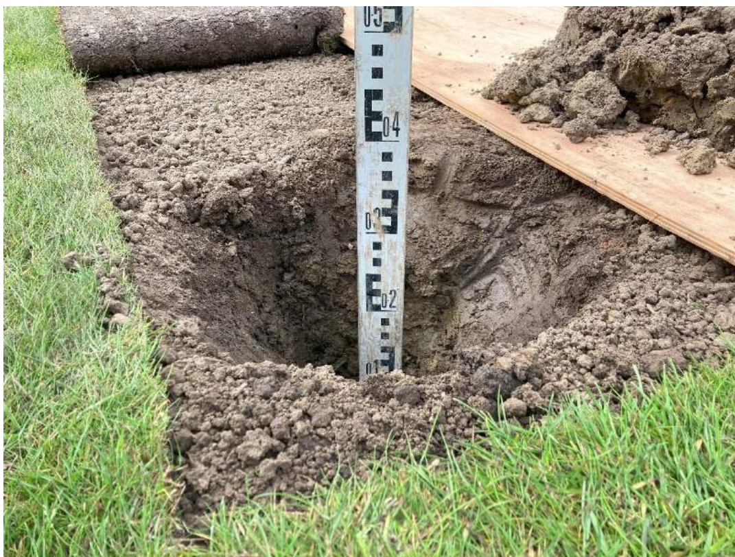
Plate 27 – HP07 GL to 0.3m bgl with 0.15m of topsoil.
