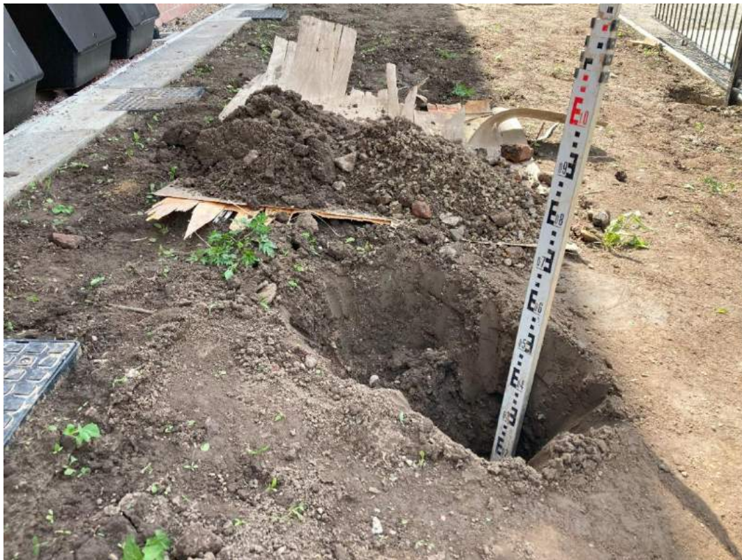
Plate 11 – HP02 GL to 0.60mbgl and arisings, with 0.15m of topsoil.
