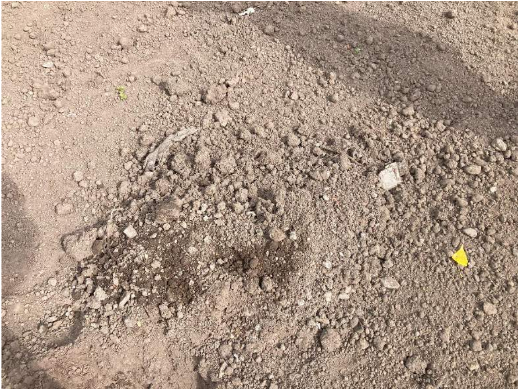
Plate 23 – HP06 GL to 0.60mbgl and arisings, with 0.20m of topsoil.
