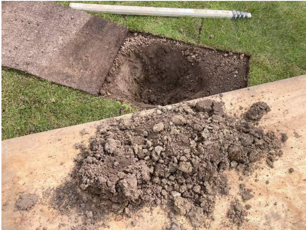
Plate 29 – HP08 GL to 0.30mbgl and arisings, with 0.15m of topsoil.
