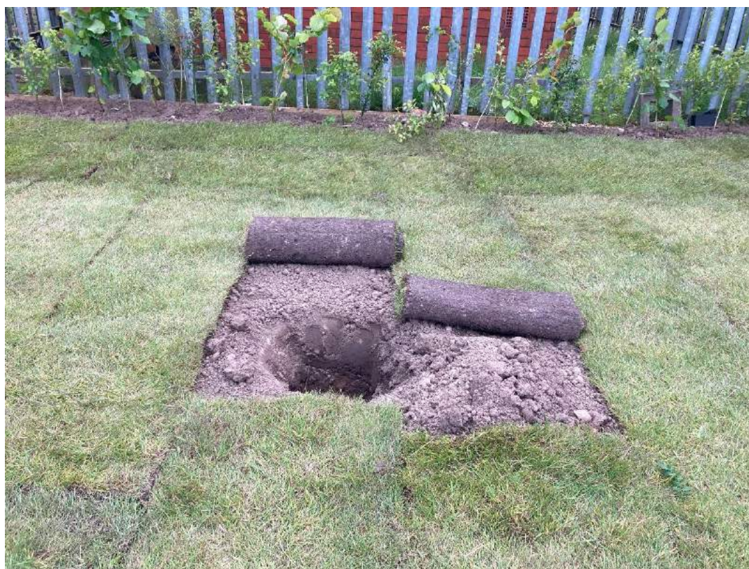
Plate 17 – HP04 GL to 0.30mbgl and arisings, with 0.15m of topsoil.
