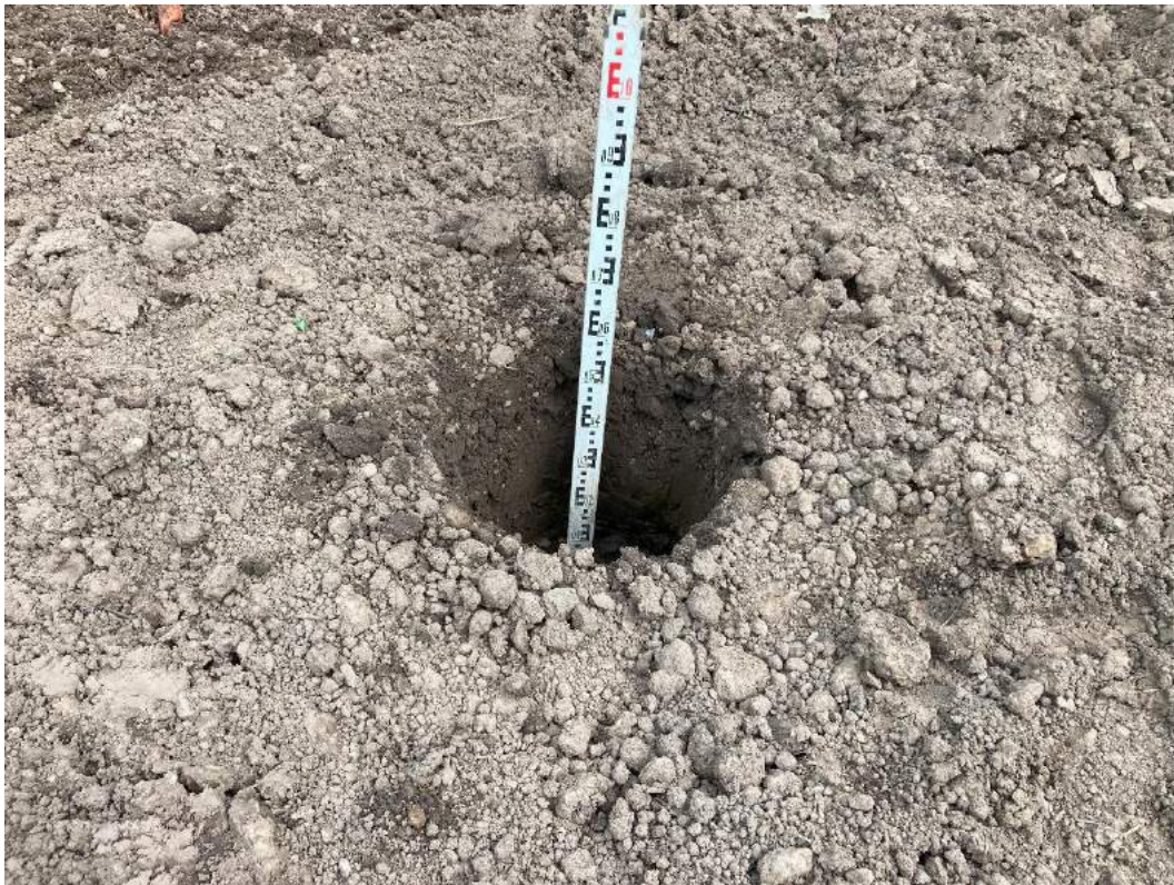
Plate 21 – HP05 GL to 0.6m bgl with 0.20m of topsoil.
