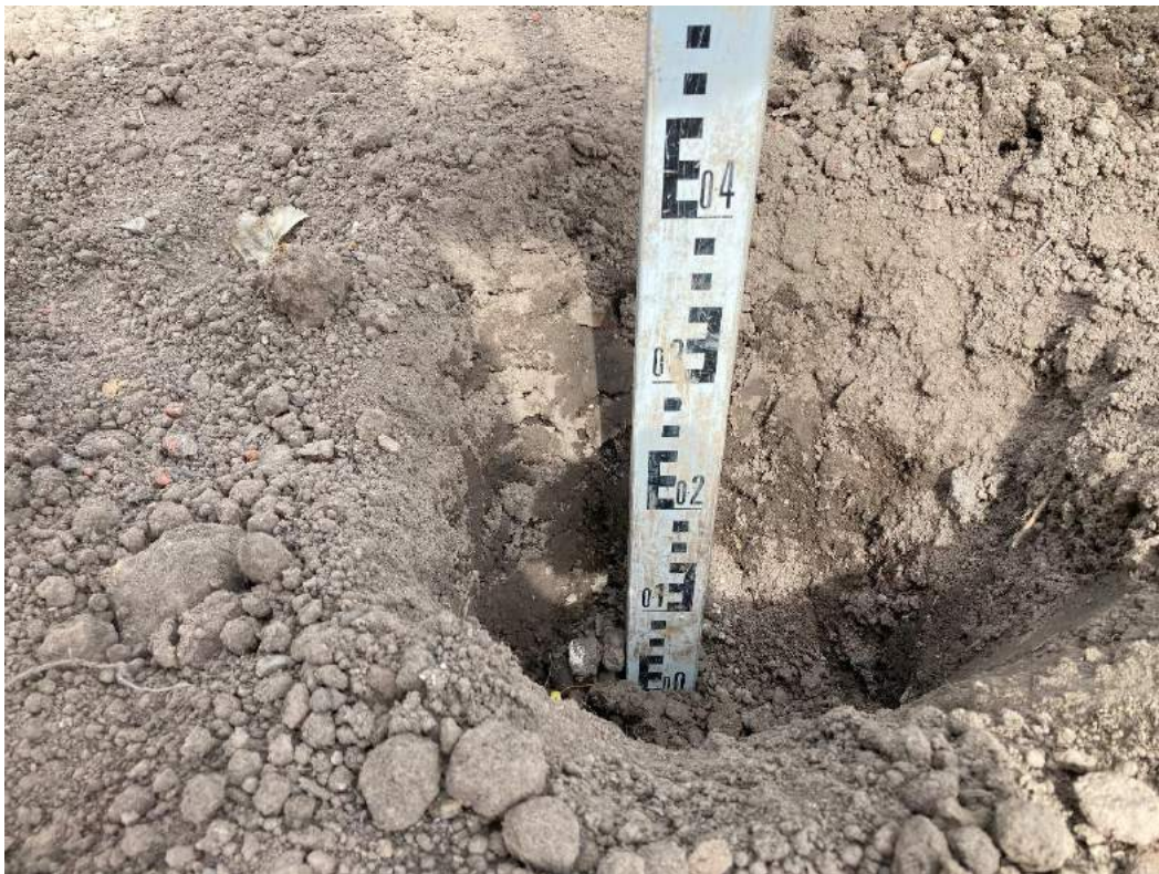
Plate 24 – HP06 GL to 0.3m bgl with 0.15m of topsoil.
