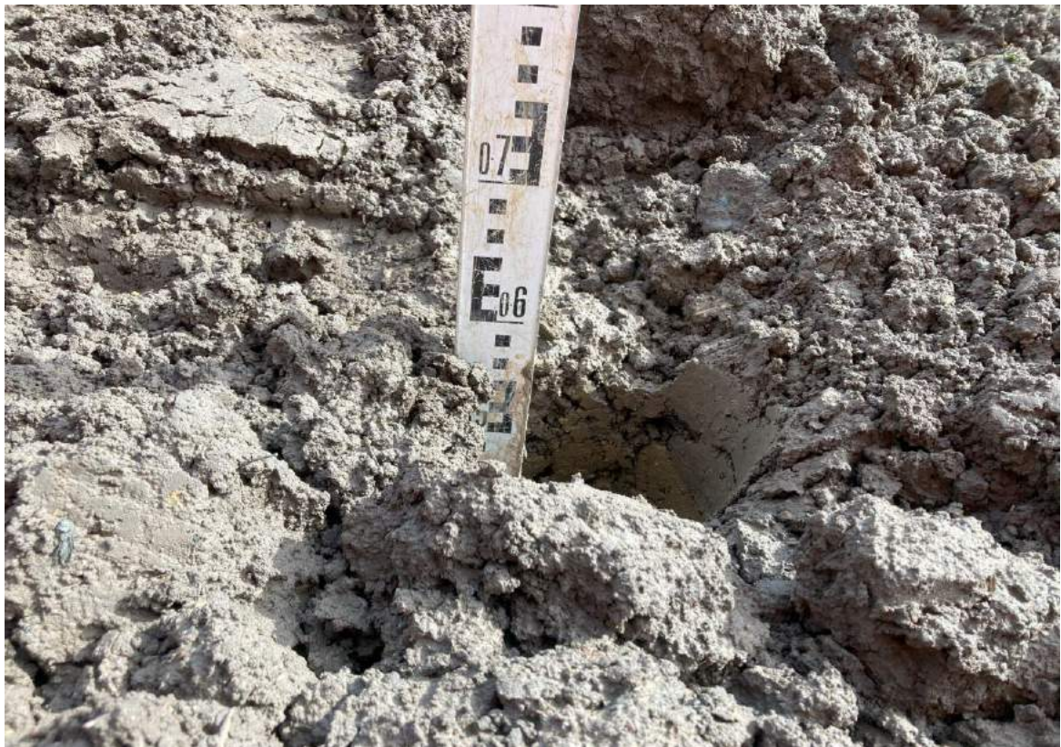
Plate 28 – Plot 5 front garden cover system GL to 0.60mbgl with 0.15m of topsoil.
