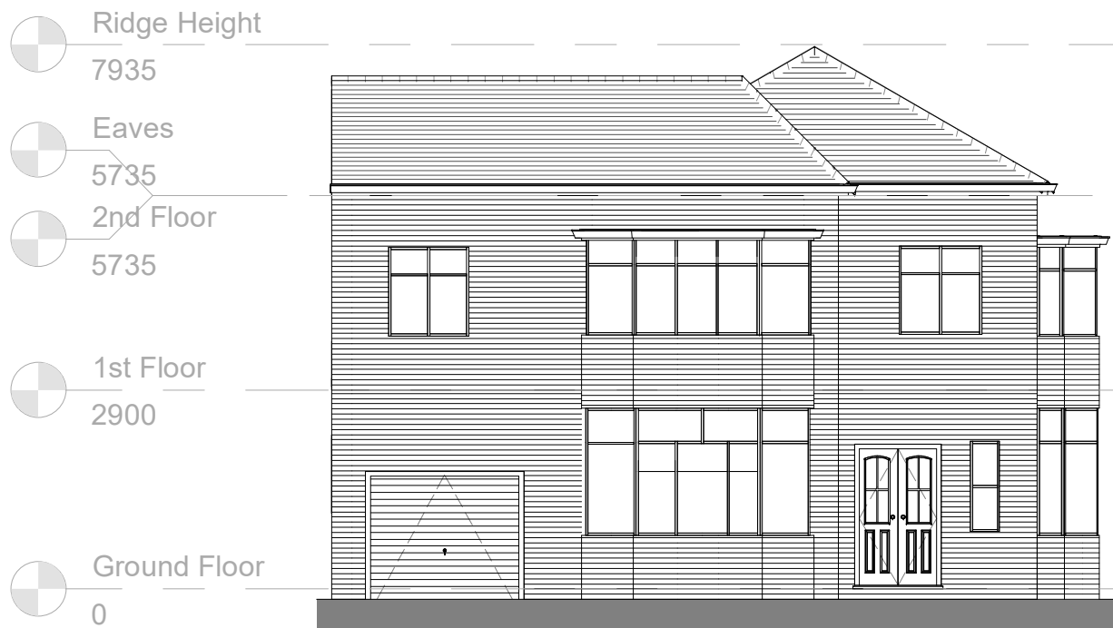
6 Existing Front Elevation 1 : 100
