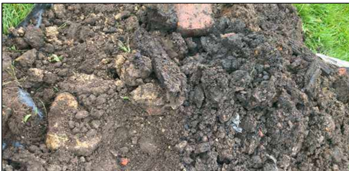
Figure 5-B: Made Ground encountered in HP01
