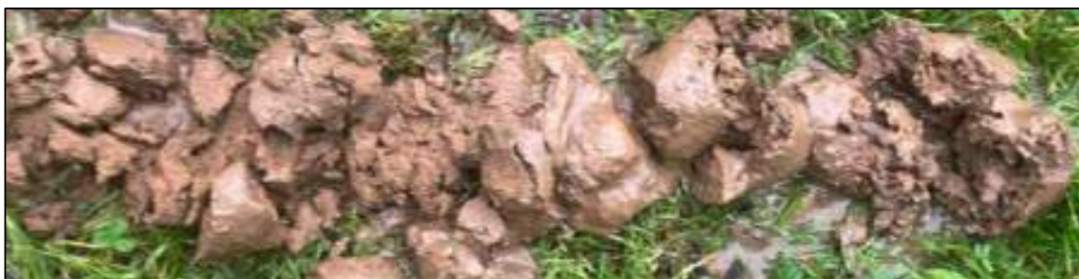
Figure 5-D: Suspected Glacial Till encountered in WLS06.
