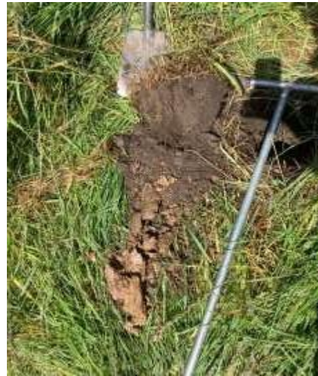
Plate 3 - SP2 - 225mm thick well-structured topsoil overlying a silty clay.
