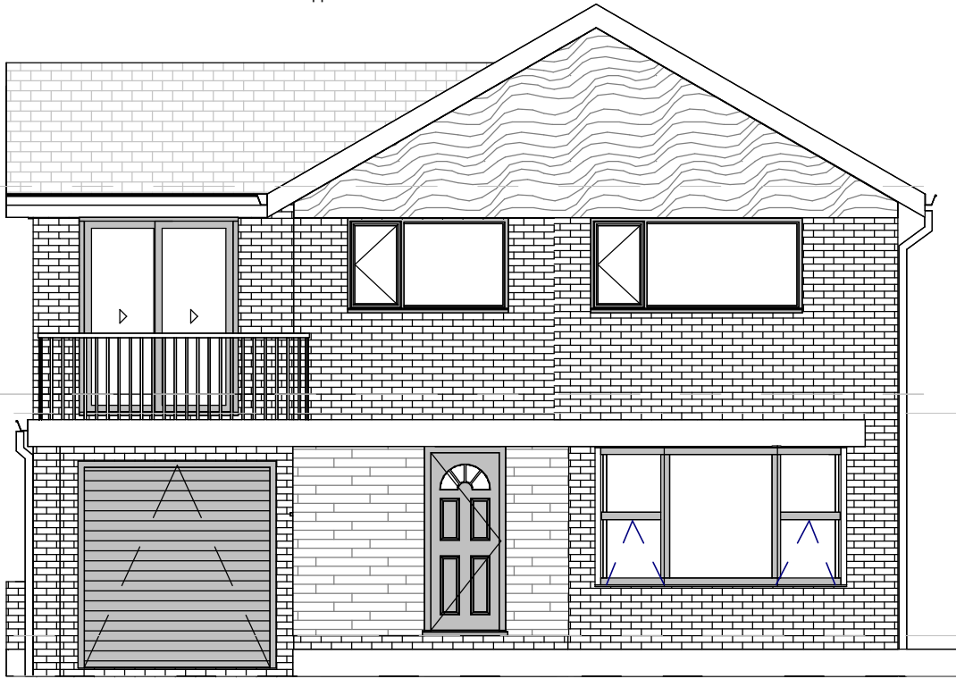
Existing Front Elevation 1 : 75
