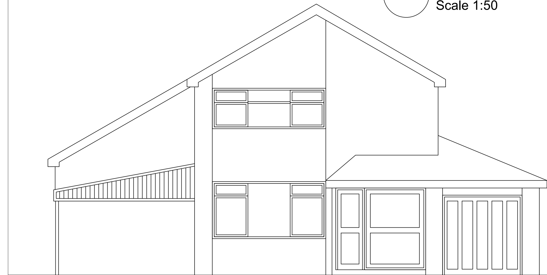
04 Existing Front Elevation Scale 1:50
