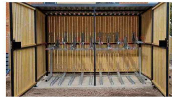
TIMBER TWO TIER BIKE SHELTER FOR MAX 12NO CYCLES. WOODEN CLADDING WITH A POWDER COATED GALVANIZED STEEL FRAME, WITH ROOF DECK AND SECURE DOUBLE GATES. LOCKING HOPE PROVIDED FOR VERTICAL BIKE STORAGE, WITH RACKS BEING STAGGERED
