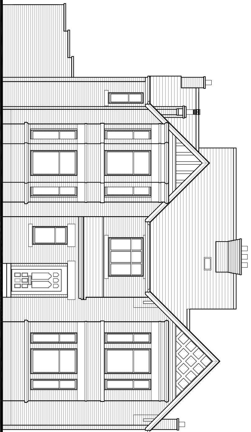
FRONT ELEVATION (SOUTHERN FACING)
