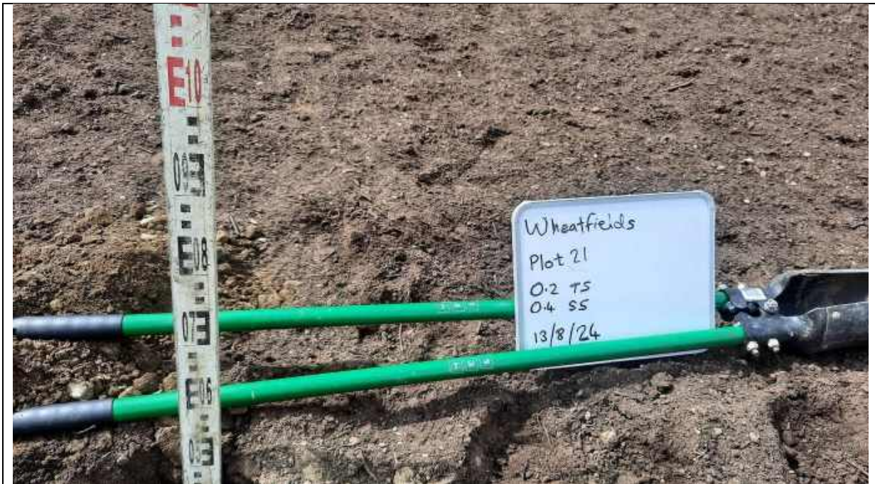
Photo 42 - Plot 21 depth validation to 0.6m.
