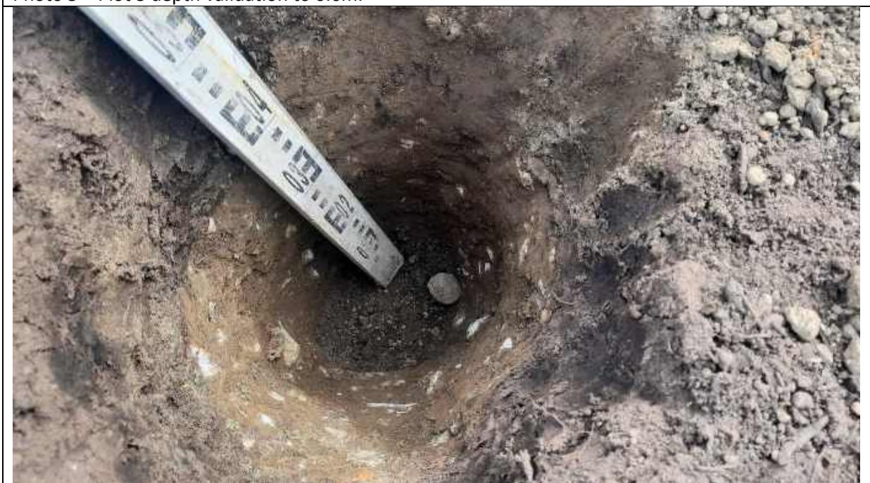
Photo 6 – Plot 3 depth validation to 0.6m.
