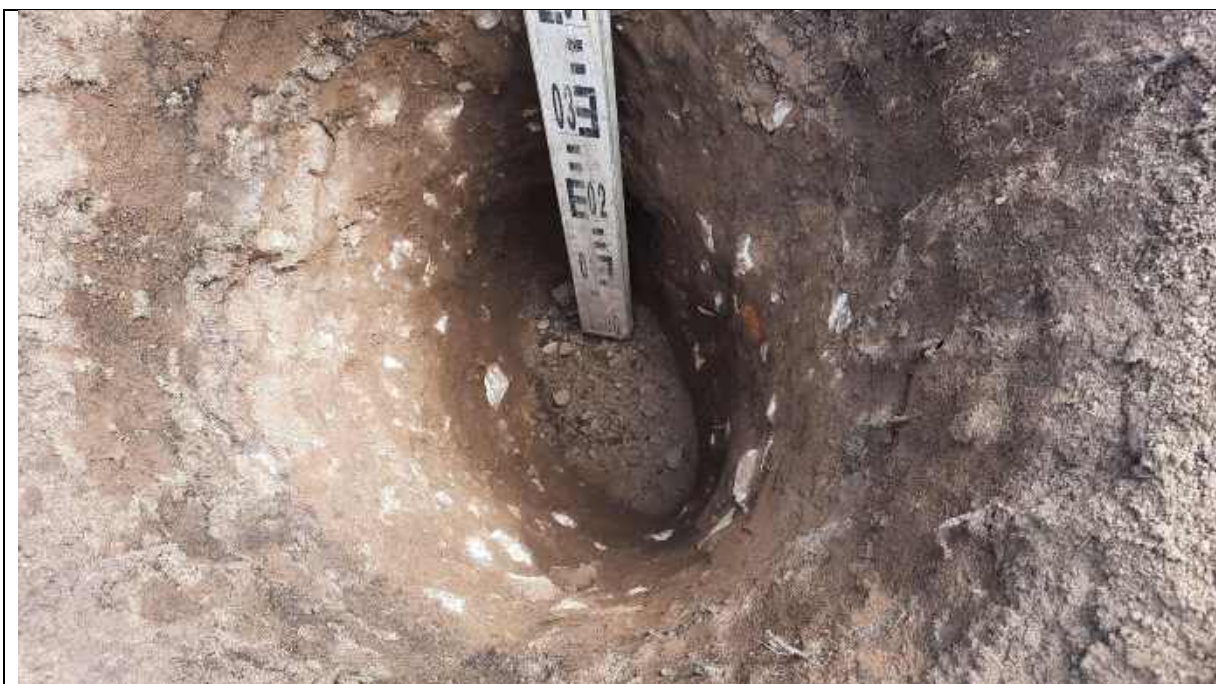
Photo 9 – Plot 4 depth validation to 0.6m.
