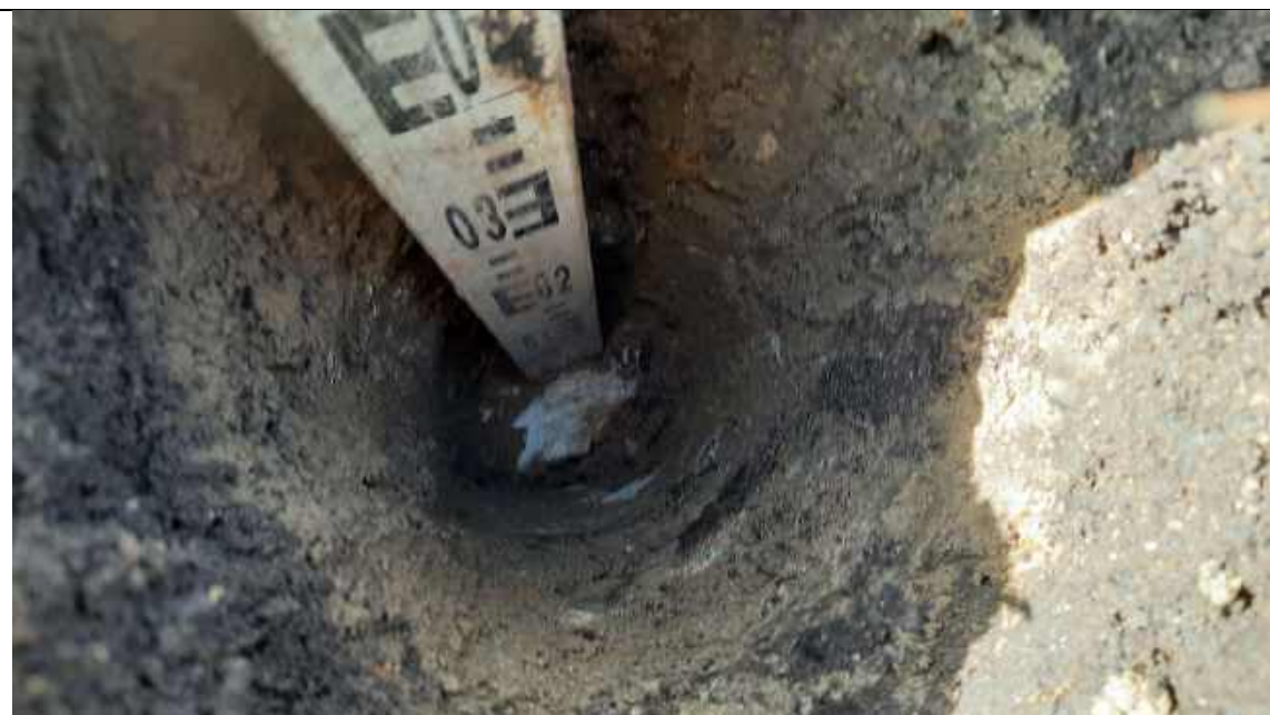
Photo 9 – Plots 25-26 apartments validation hole to 0.6m.
