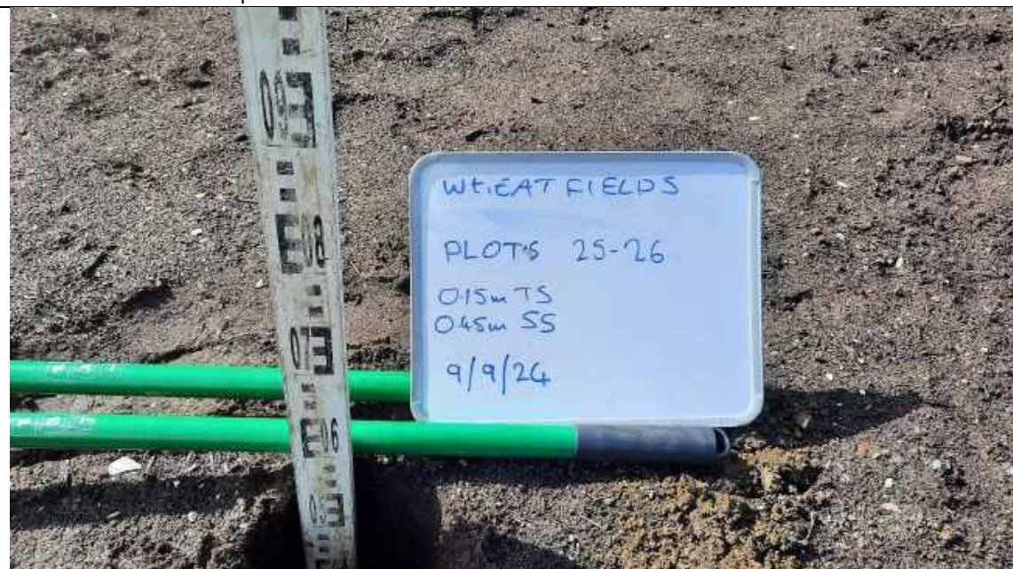
Photo 8 – Plots 25-26 apartments validation hole to 0.6m.
