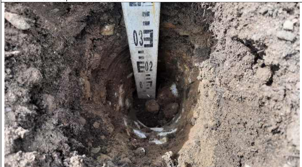
Photo 43 - Plot 21 depth validation to 0.6m.
