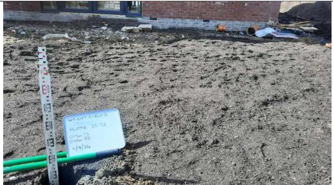
Photo 7 – Plots 25-26 apartments validation hole to 0.6m.
