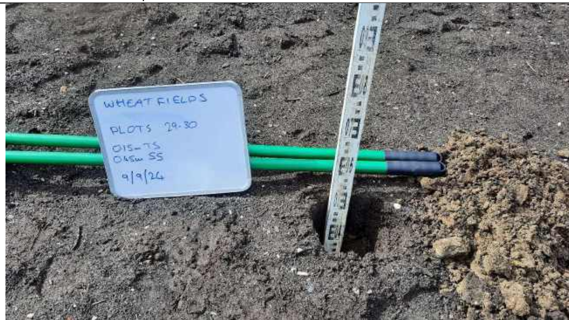
Photo 14 – Plots 29-30 apartments validation hole to 0.6m.
