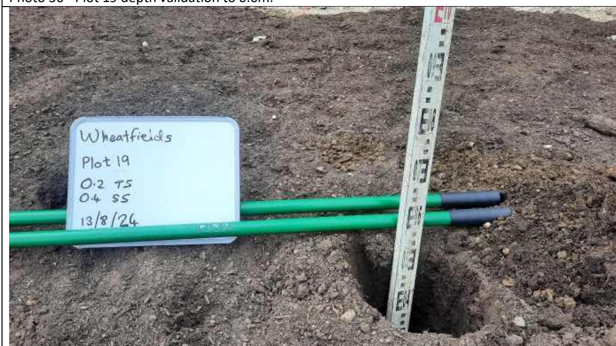
Photo 37 - Plot 19 depth validation to 0.6m.
