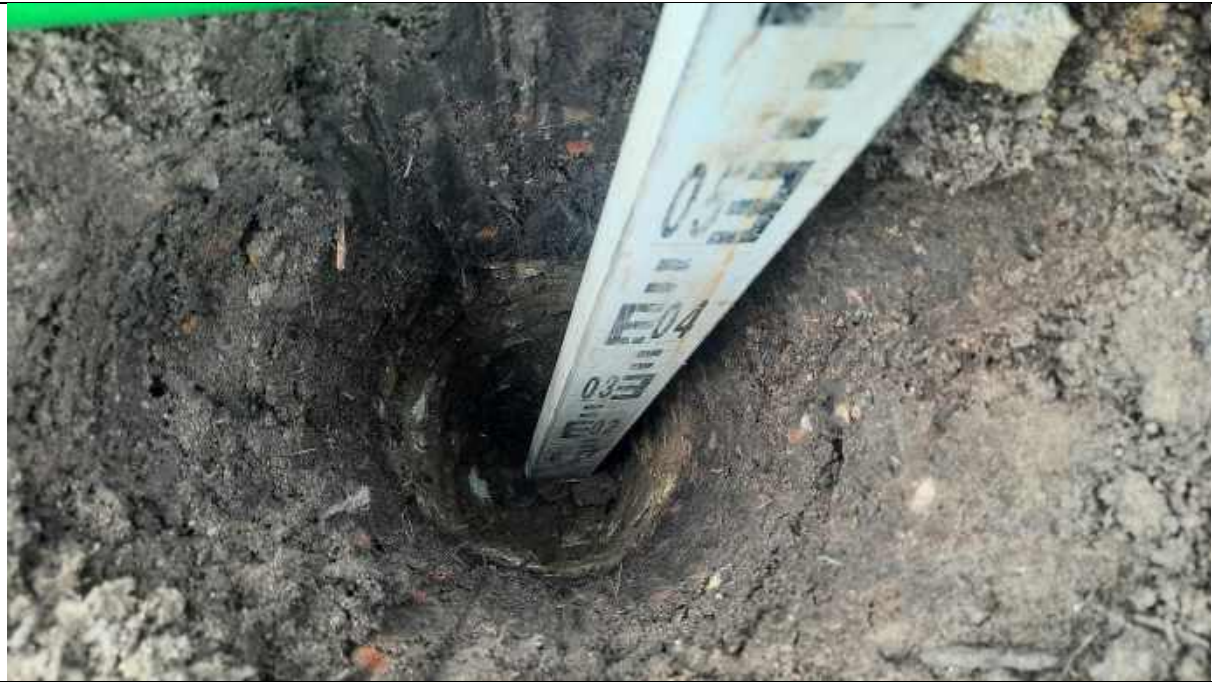
Photo 40 - Plot 20 depth validation to 0.6m.
