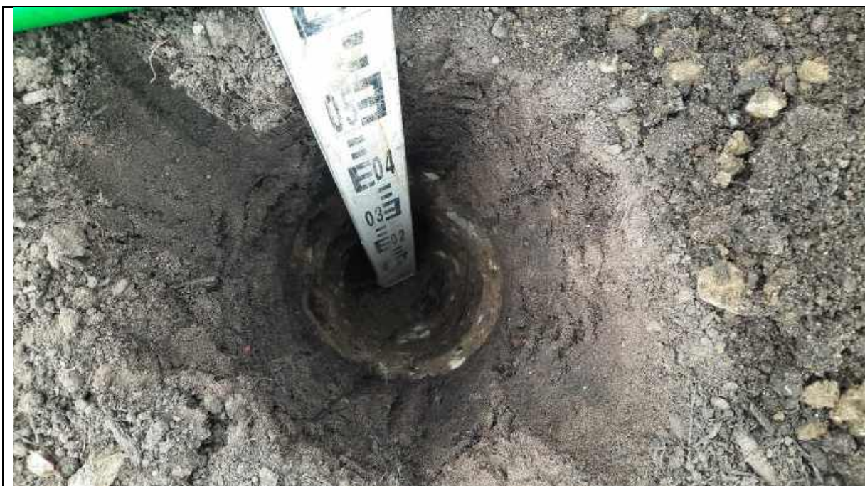
Photo 38 - Plot 20 depth validation to 0.6m.
