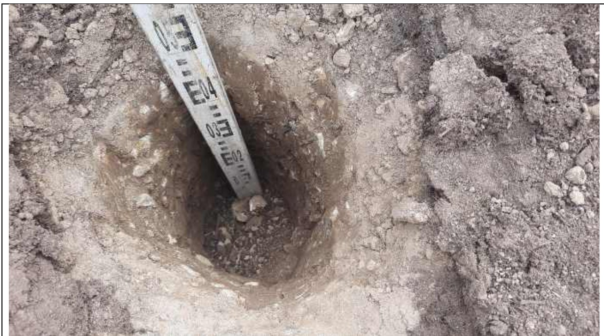
Photo 31 - Plot 12 depth validation to 0.6m.
