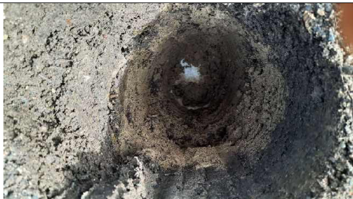
Photo 15 – Plots 29-30 apartments validation hole to 0.6m.
