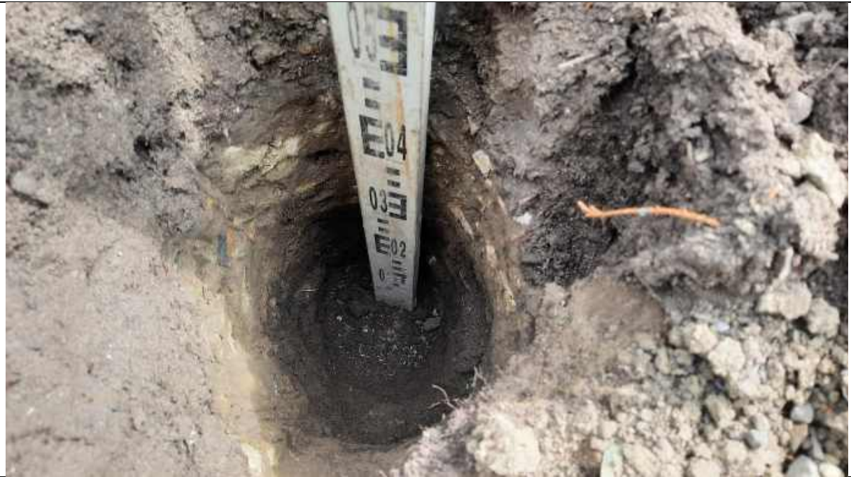
Photo 17 – Plot 7 depth validation to 0.6m.
