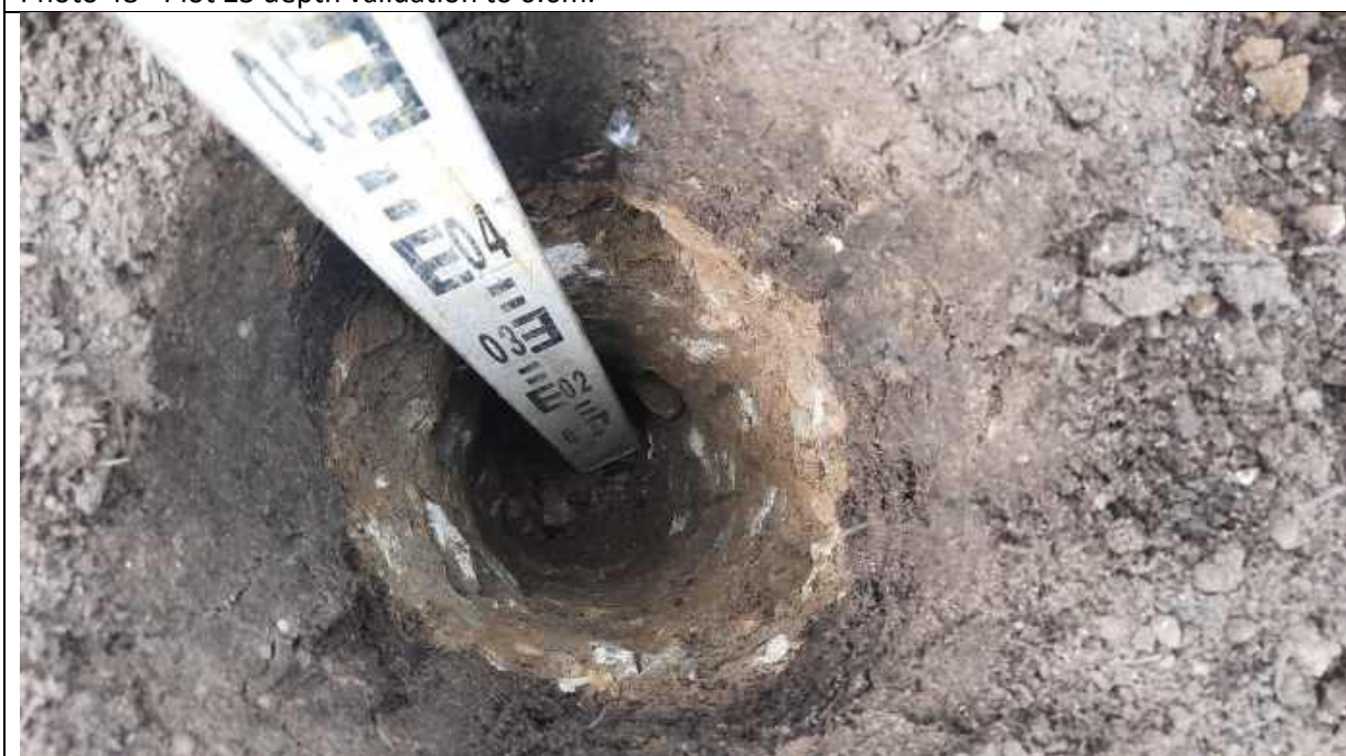
Photo 49 - Plot 23 depth validation to 0.6m.
