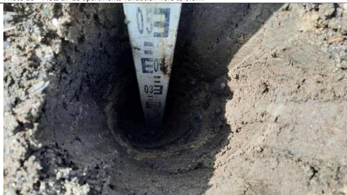
Photo 12 – Plots 27-28 apartments validation hole to 0.6m.
