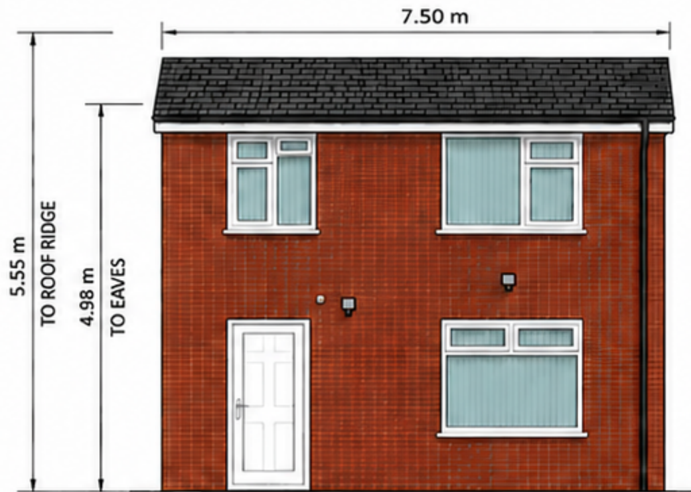
EXISTING REAR ELEVATION 1:100
