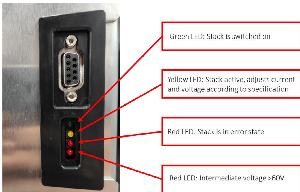
Figure 18: Status indication of Power-Stack
