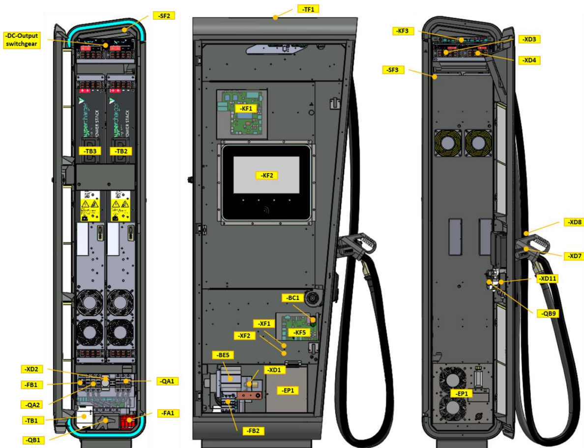
Figure 13: Internal view hypercharger HYC_150 (service-, display-, charging cable side)
