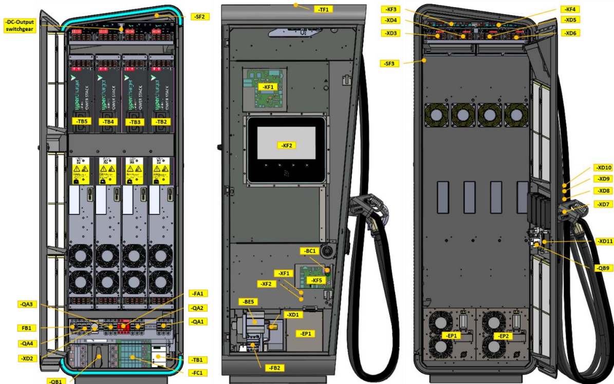
Figure 14: Internal view hypercharger HYC_300 (service-, display- and charging cable-side)
