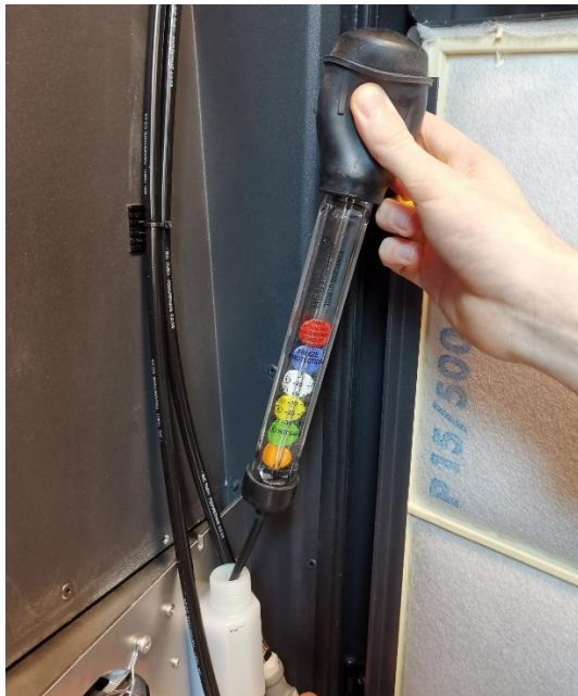
Figure 84: Check the coolant concentration using a refractometer
