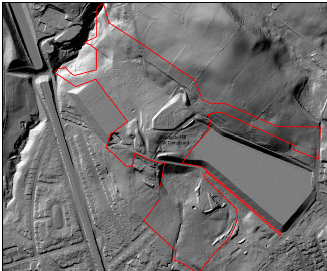
Figure 7 – Lidar imagery of the site identifying areas of made ground.
