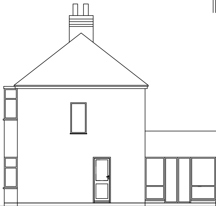
EXISTING SIDE ELEVATION
