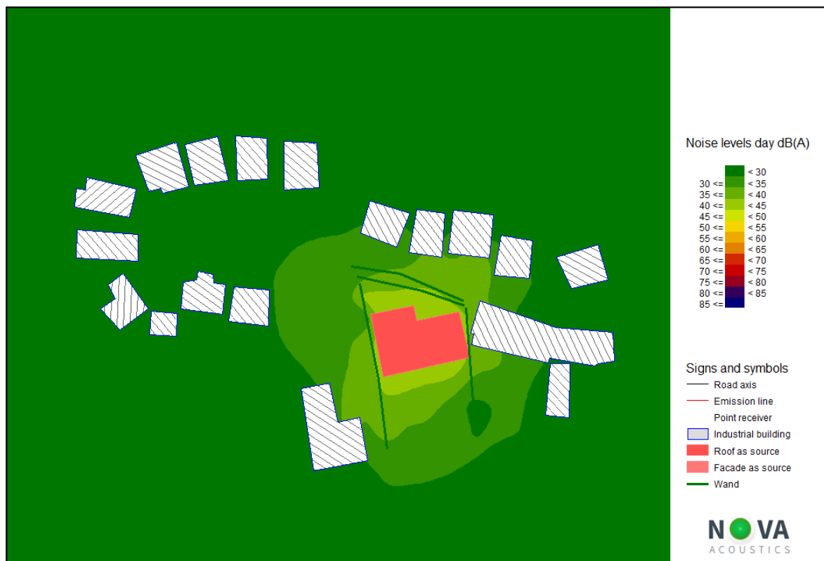
Figure 3.0 – Specific Sound Level Map of Internal Breakout with the Recommended Mitigation.
