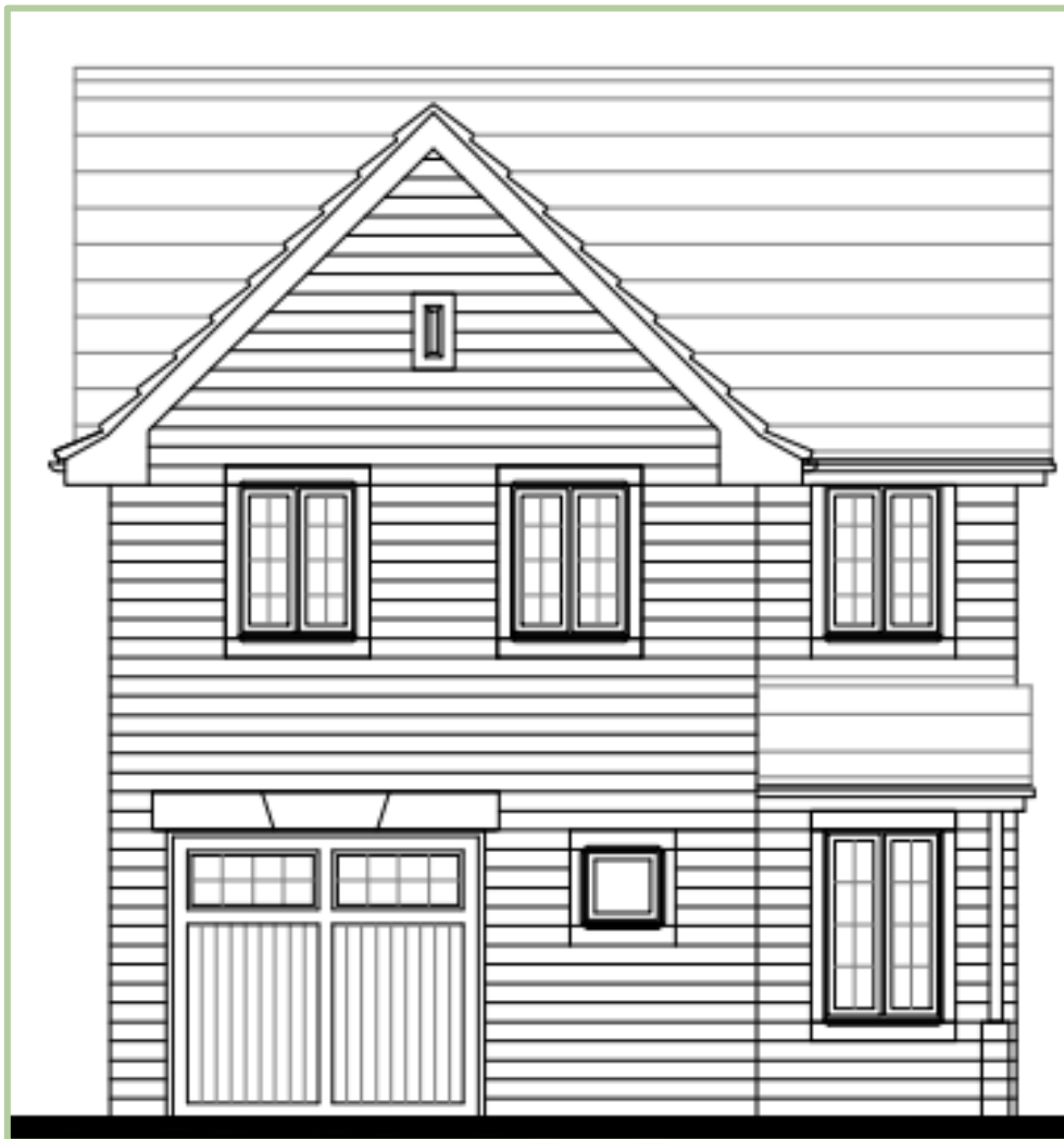
Figure 2.5 – Proposed Front Elevation – House Type Whalley
