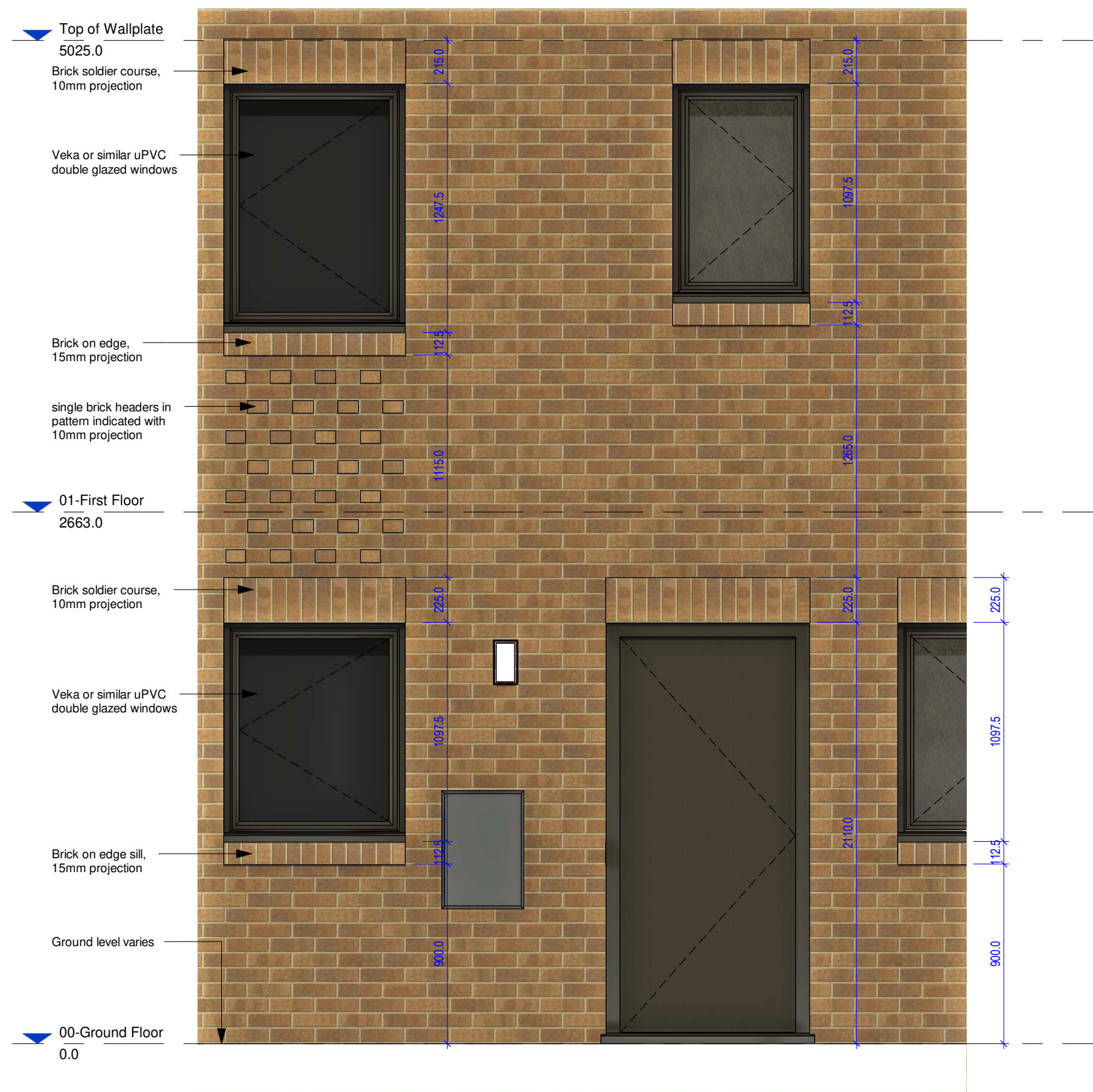
Side Elevation 4 Brick Detailing
