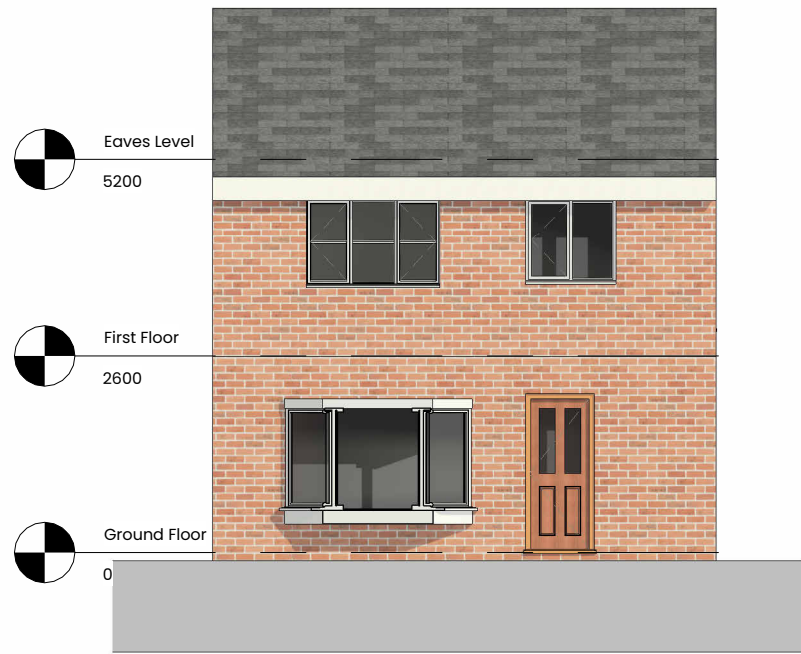
1 Existing Front Elevation 1 : 100
