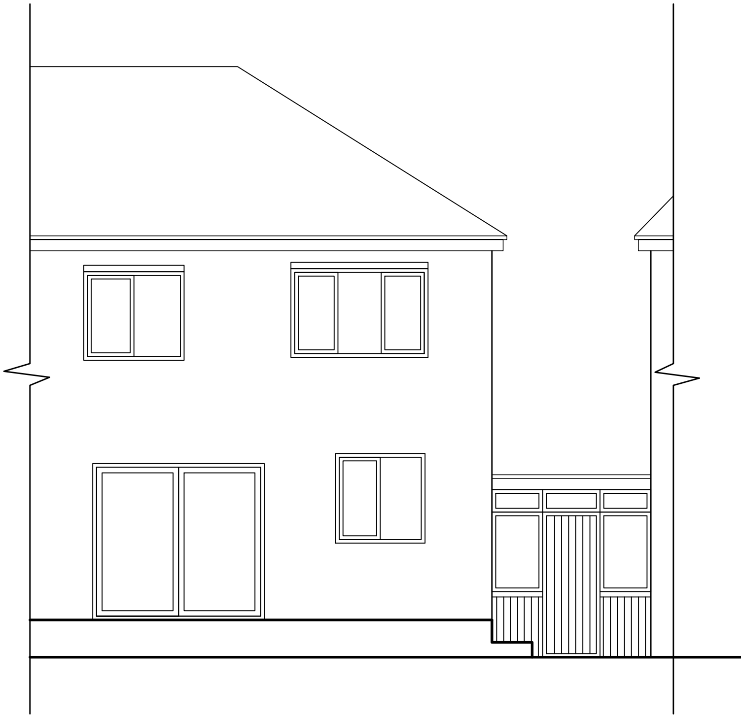
03 Existing Rear Elevation Scale 1:50
