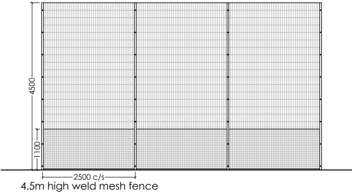
PROPOSED FENCE ELEVATION 1:100
