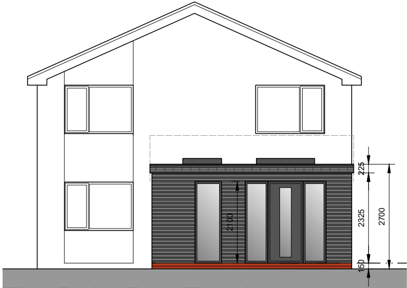
West Facing Front Elevation
