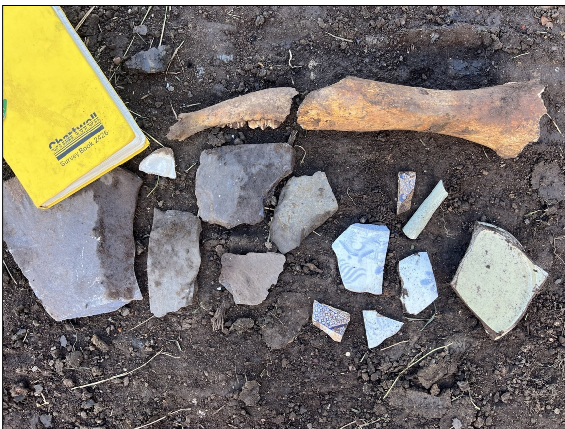
002 Evidence of made ground from TT07 and TT08
