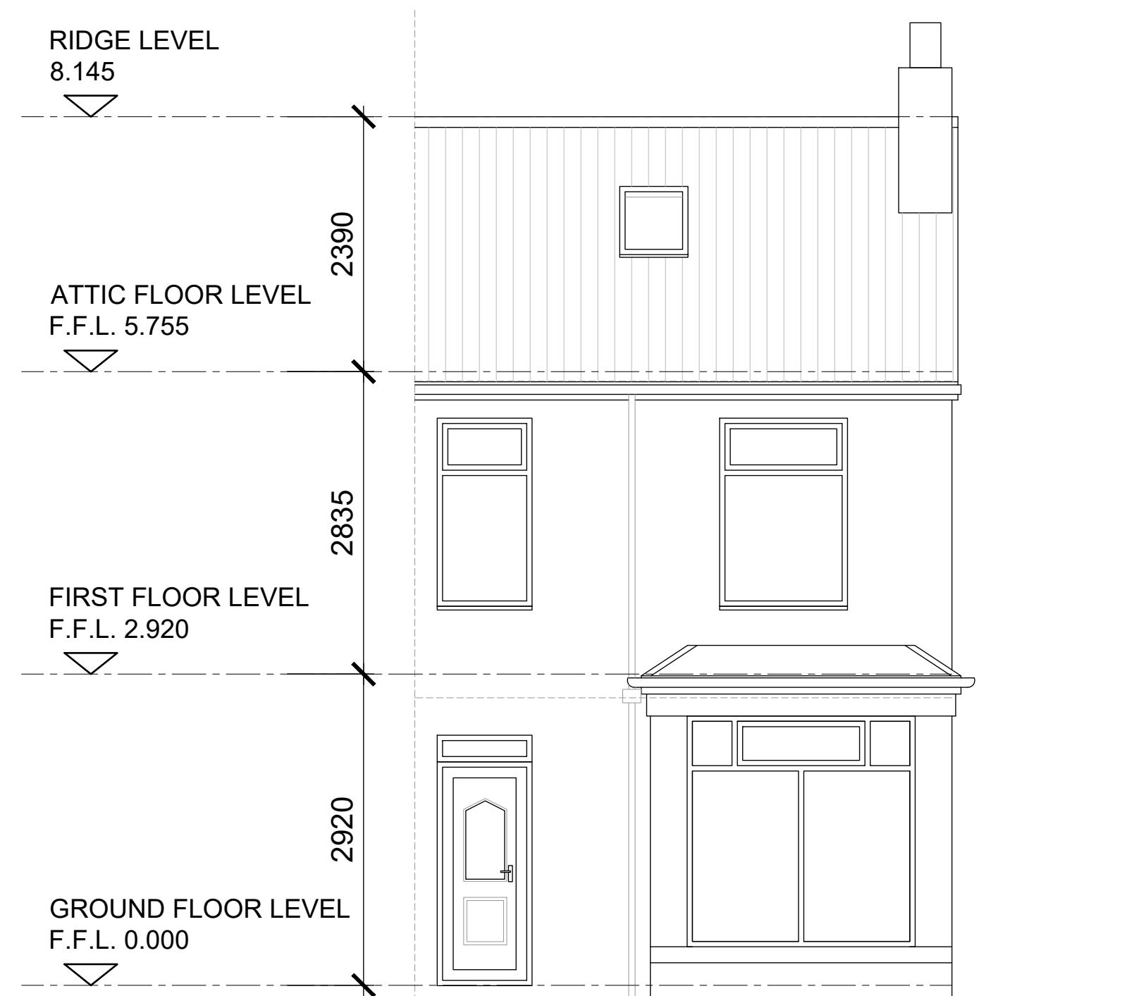
EXISTING FRONT ELEVATION
