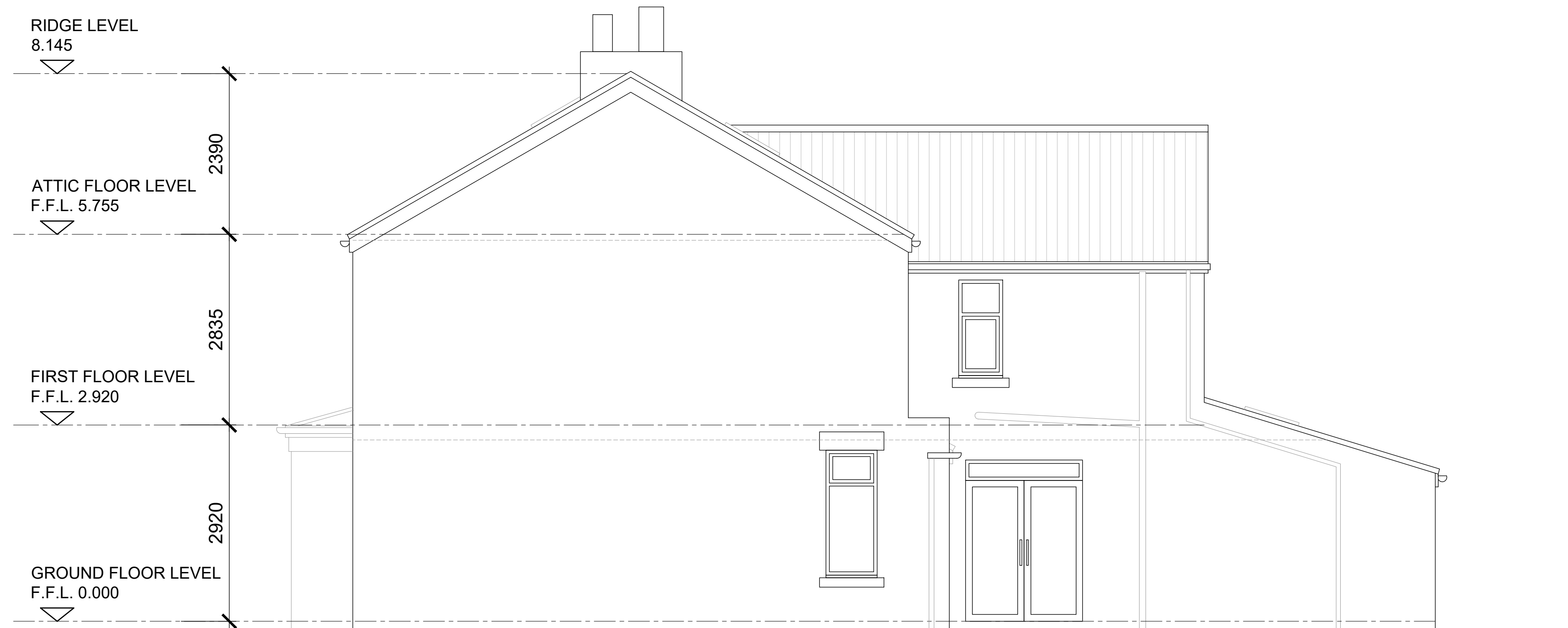
EXISTING SIDE ELEVATION
