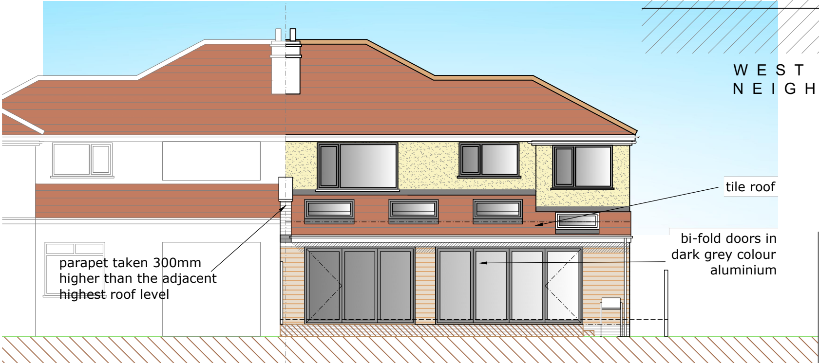
SOUTH EAST (REAR) ELEVATION
