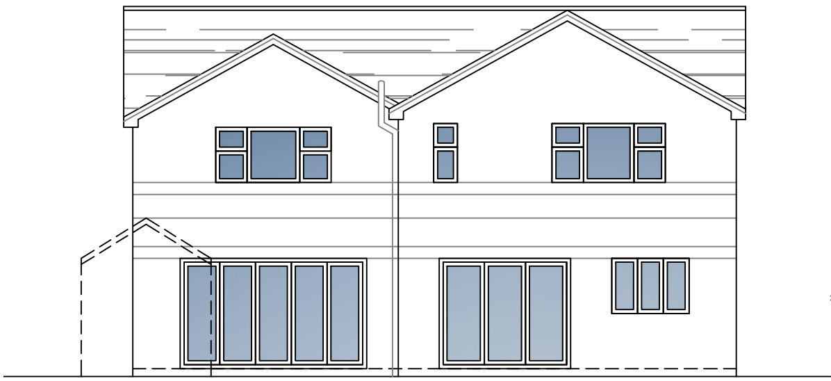
EXISTING REAR ELEVATION scale - 1:100
