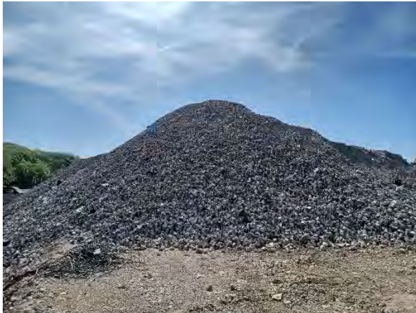
30.04.25 – Crushed concrete stockpile
