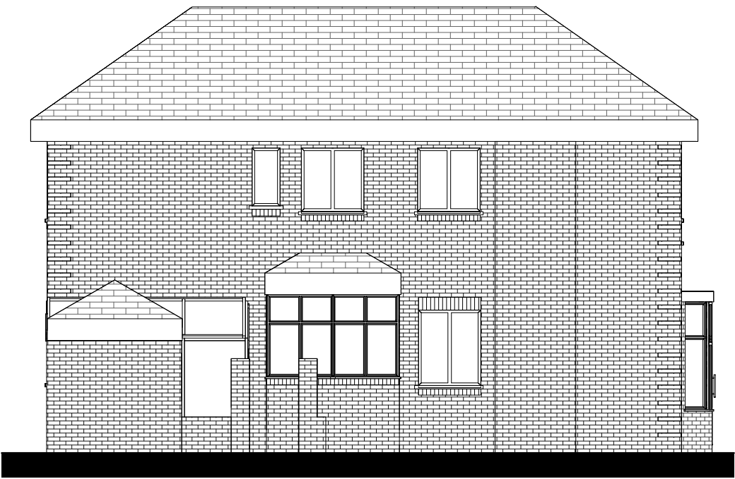
4 Existing Rear Side Elevation 1 : 100
