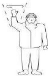
HOIST Clench and unclench fingers to 'inch' load
