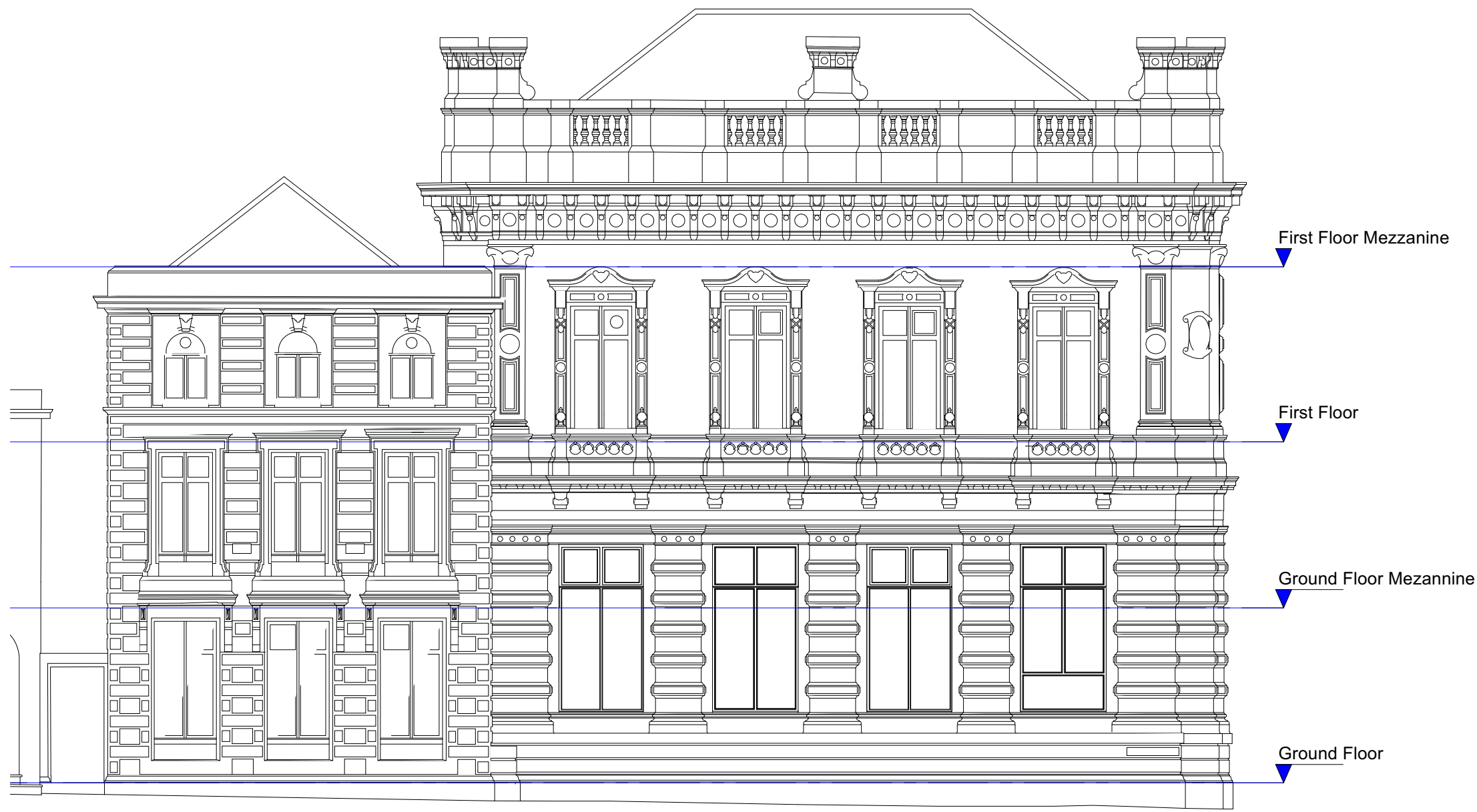
Side Elevation (Bank Street) As Existing Scale 1:100
