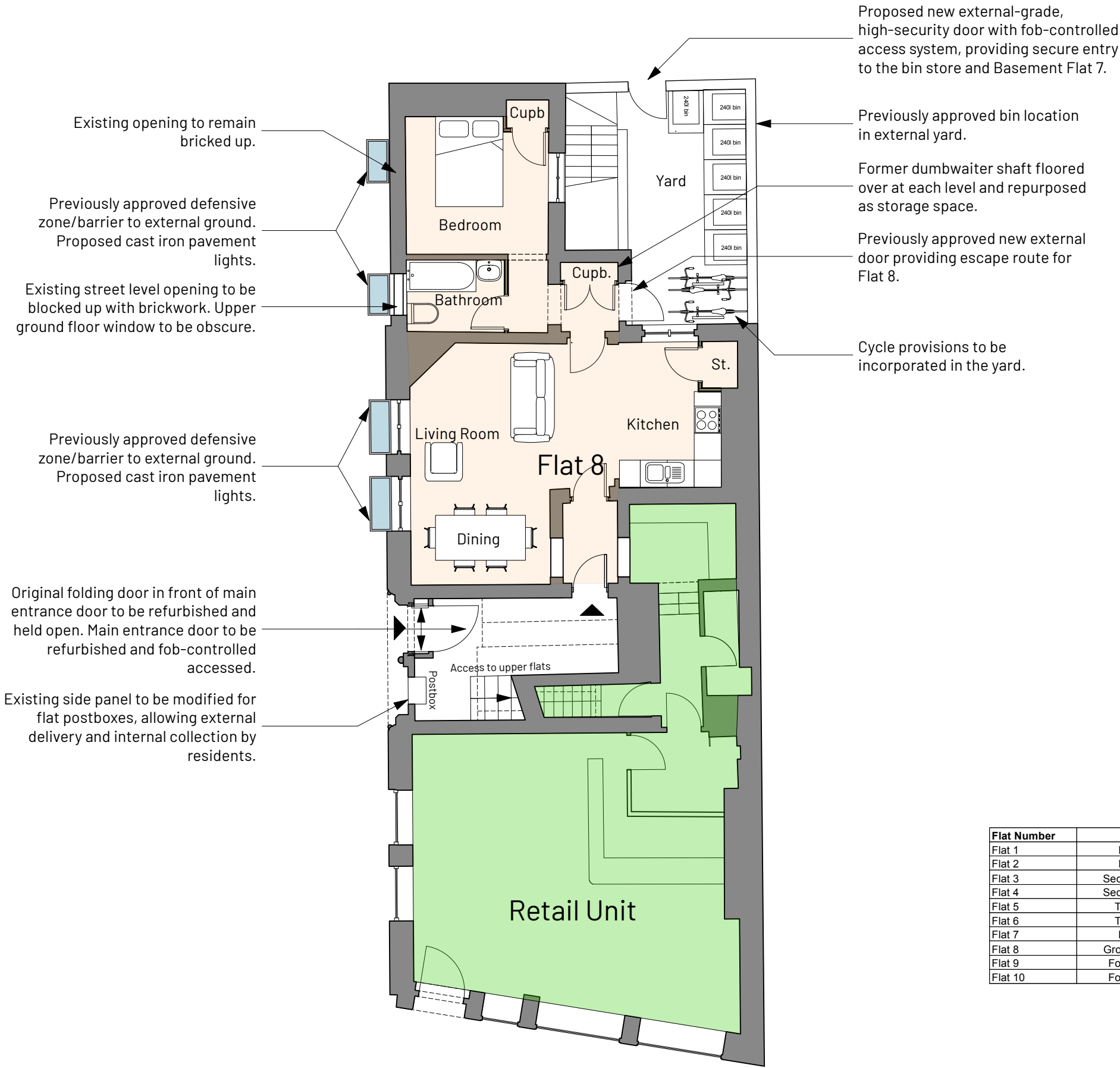
1 Ground Floor Plan Proposed Scale: 1:100
