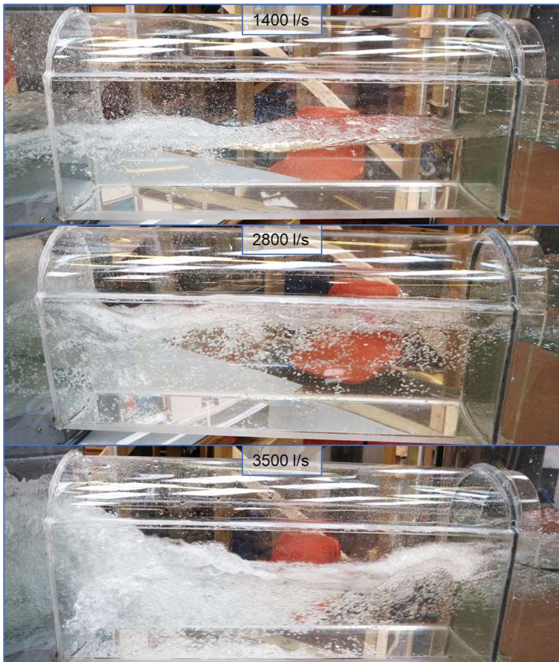
Image 4.16 – Flow conditions within the Outlet Culvert at flow rates of 1400 l/s, 2800 l/s and 3500 l/s
