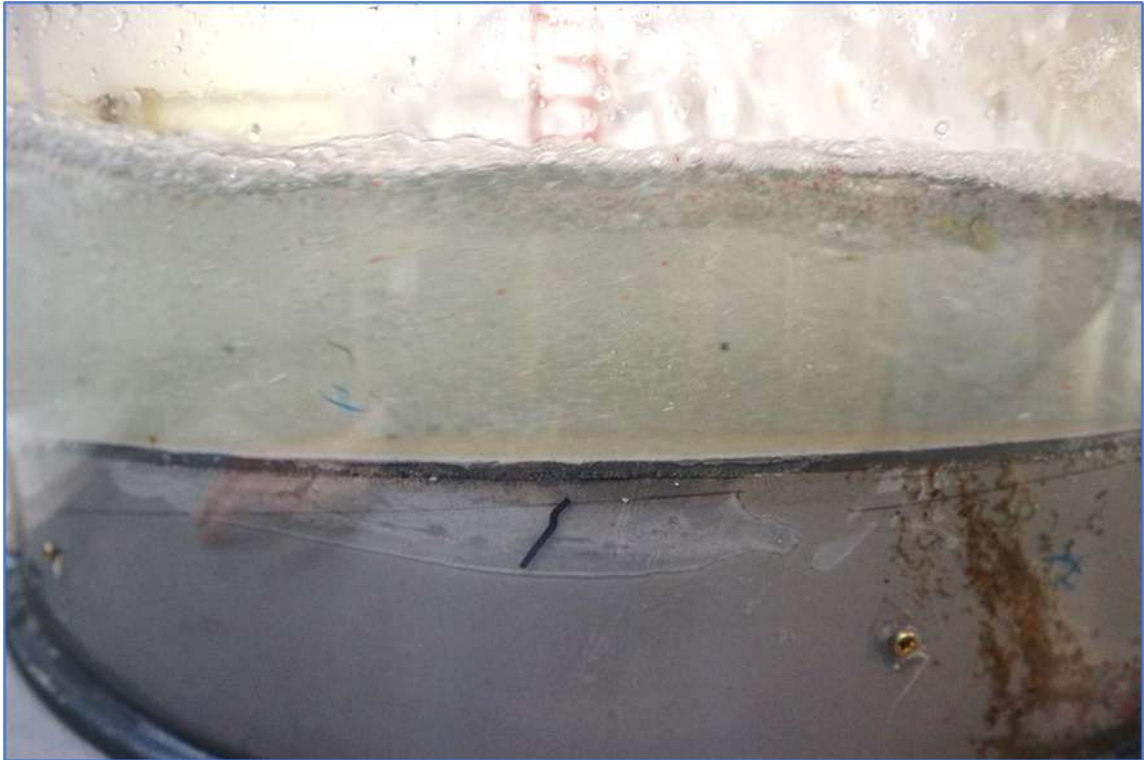
Image 4.23– Absence of solids at Level 5 at a flow rate of 1400 l/s
