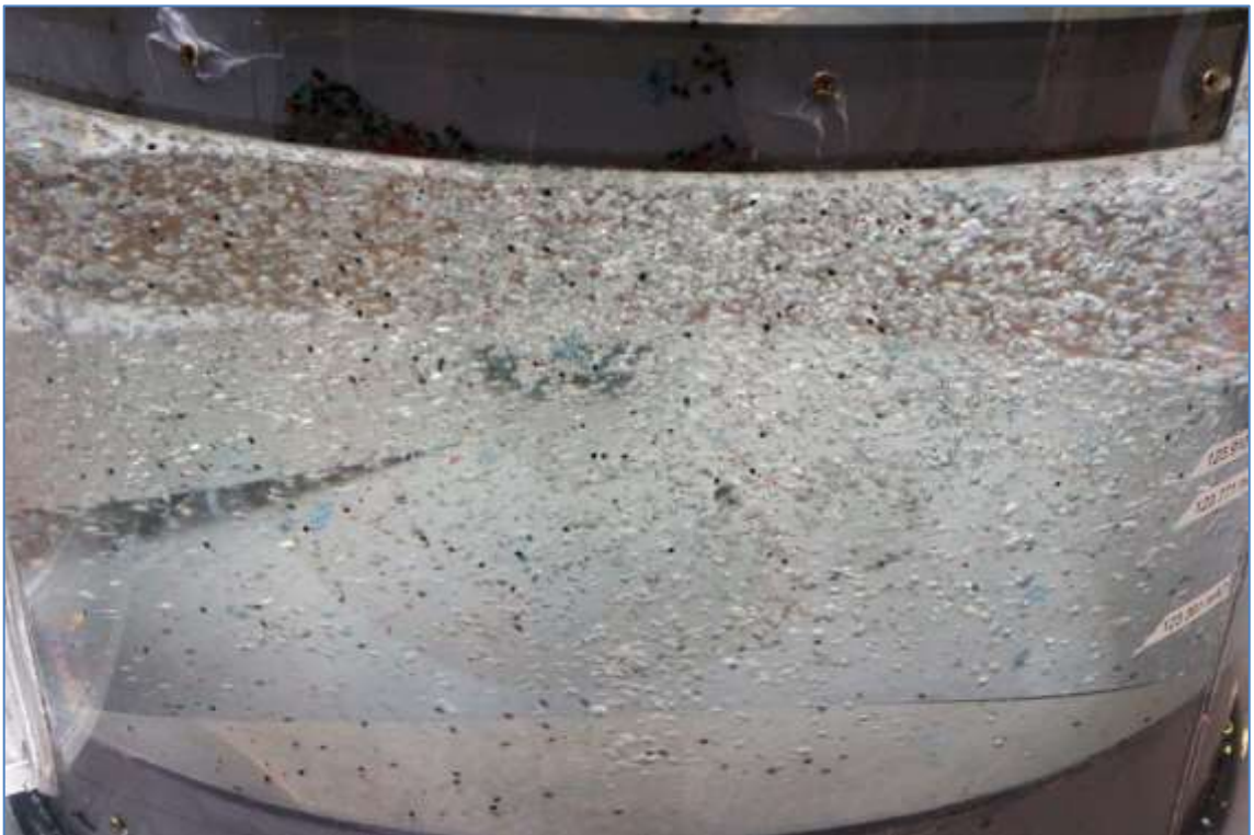
Image 4.19 – Solids in suspension at Level 5 at a flow rate of 7500 l/s
