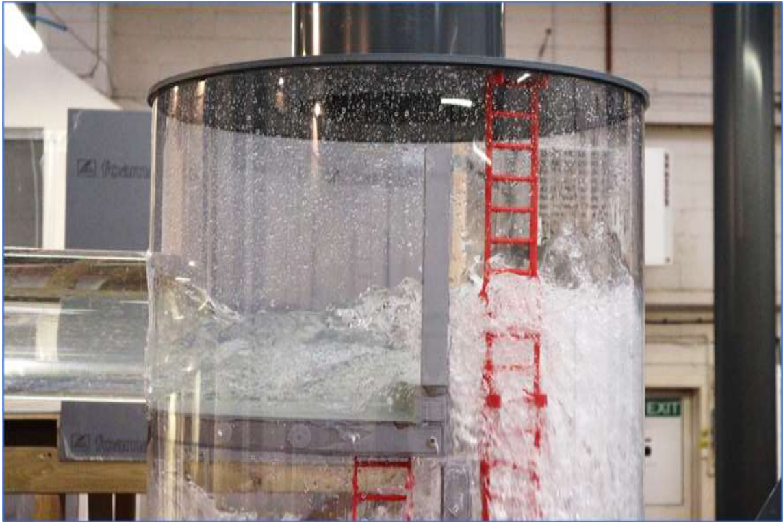
Image 4.08 – Flow conditions at Level 1 at a flow rate of 5670 l/s
