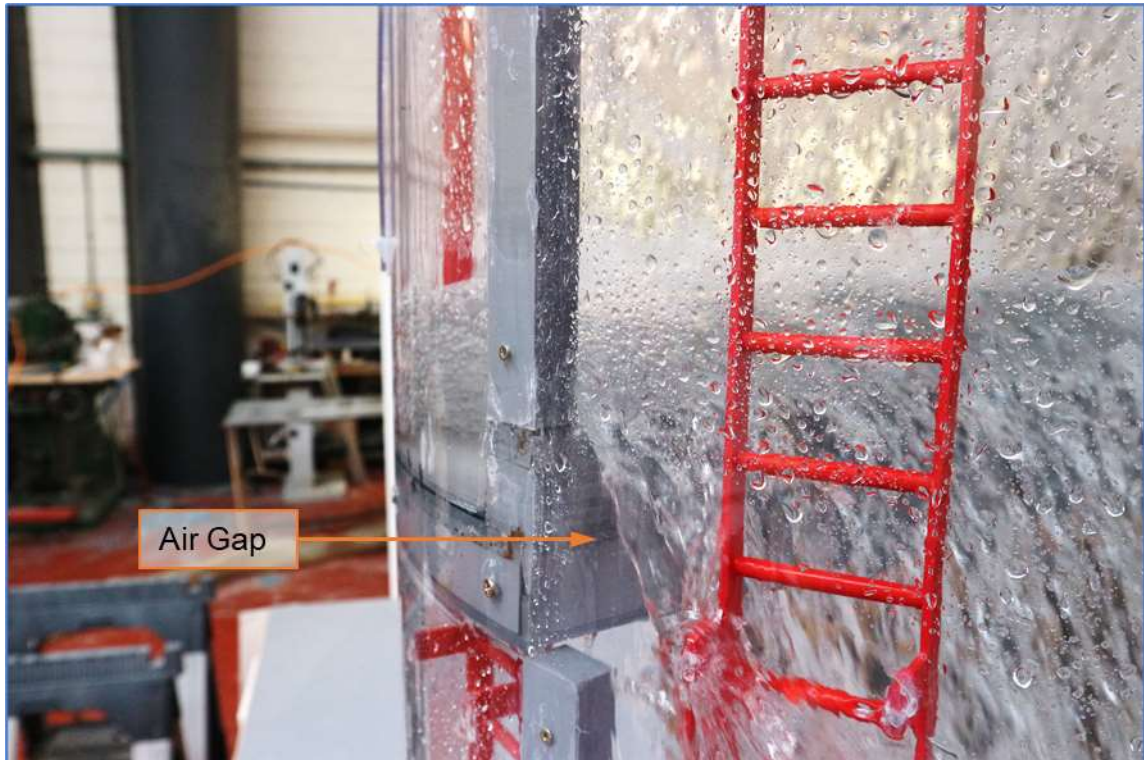
Image 4.14 – Flow deflection column effects at Level 3 at a flow rate of 1400 l/s
