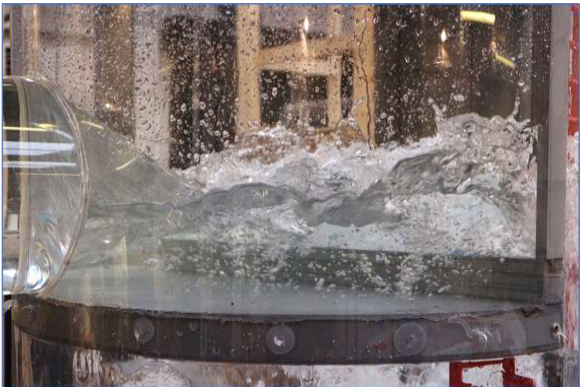
Image 4.20 – Absence of solids at Level 1 at a flow rate of 5670 l/s
