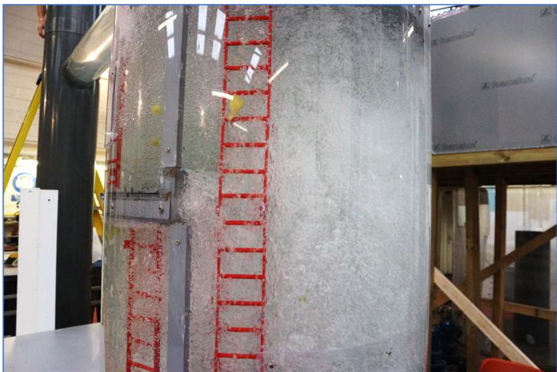
Image 4.22 – Highly buoyant solids at Level 2 at a flow rate of 5670 l/s
