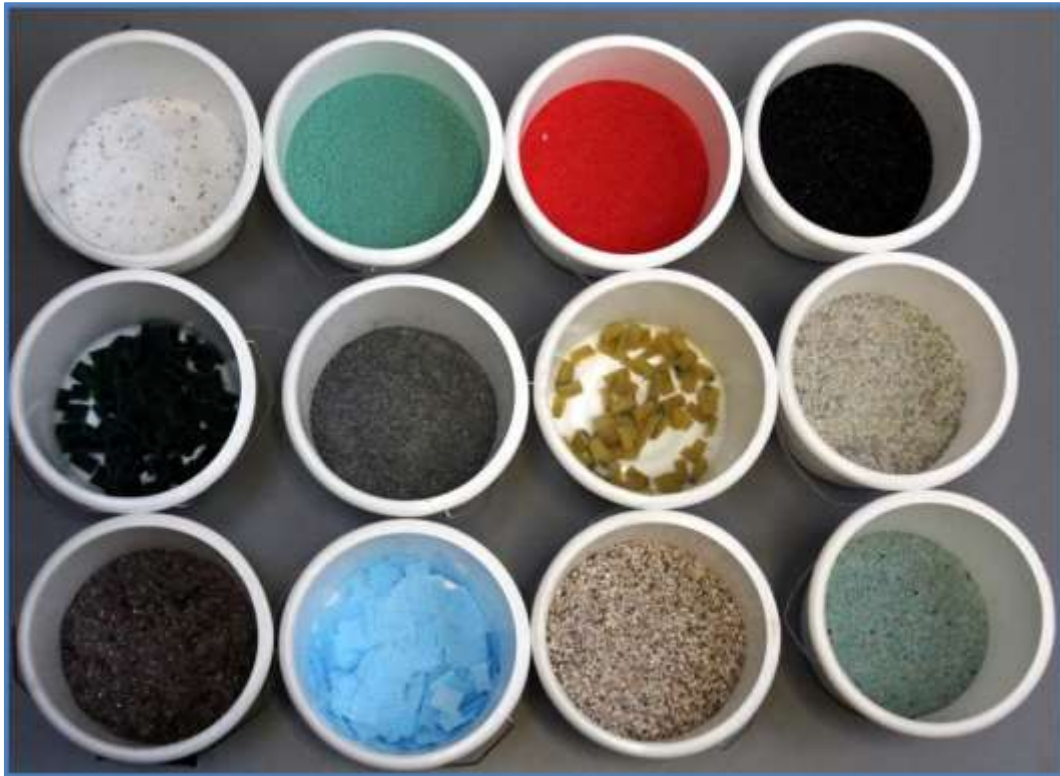
Image 1.05 - Typical representation of modelled solids introduced into the Bury drop structure MH6 model
