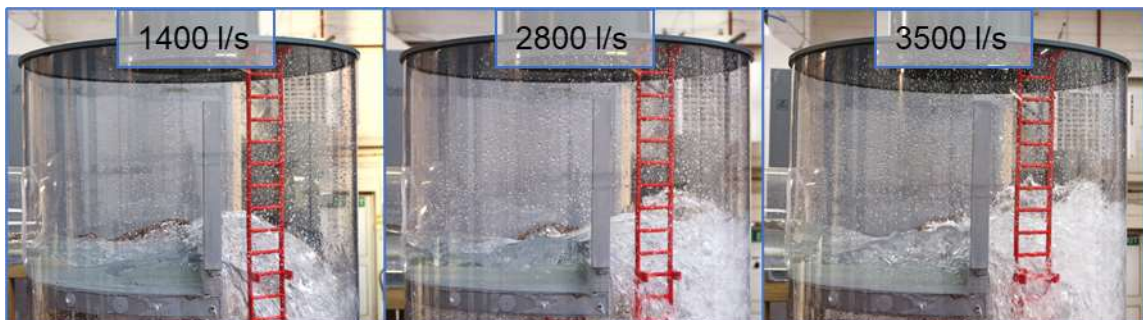
Image 4.12 – Flow conditions at Level 1 of Bury Drop Structure MH6 at flow rates of 1400 l/s, 2800 l/s and 3500 l/s
