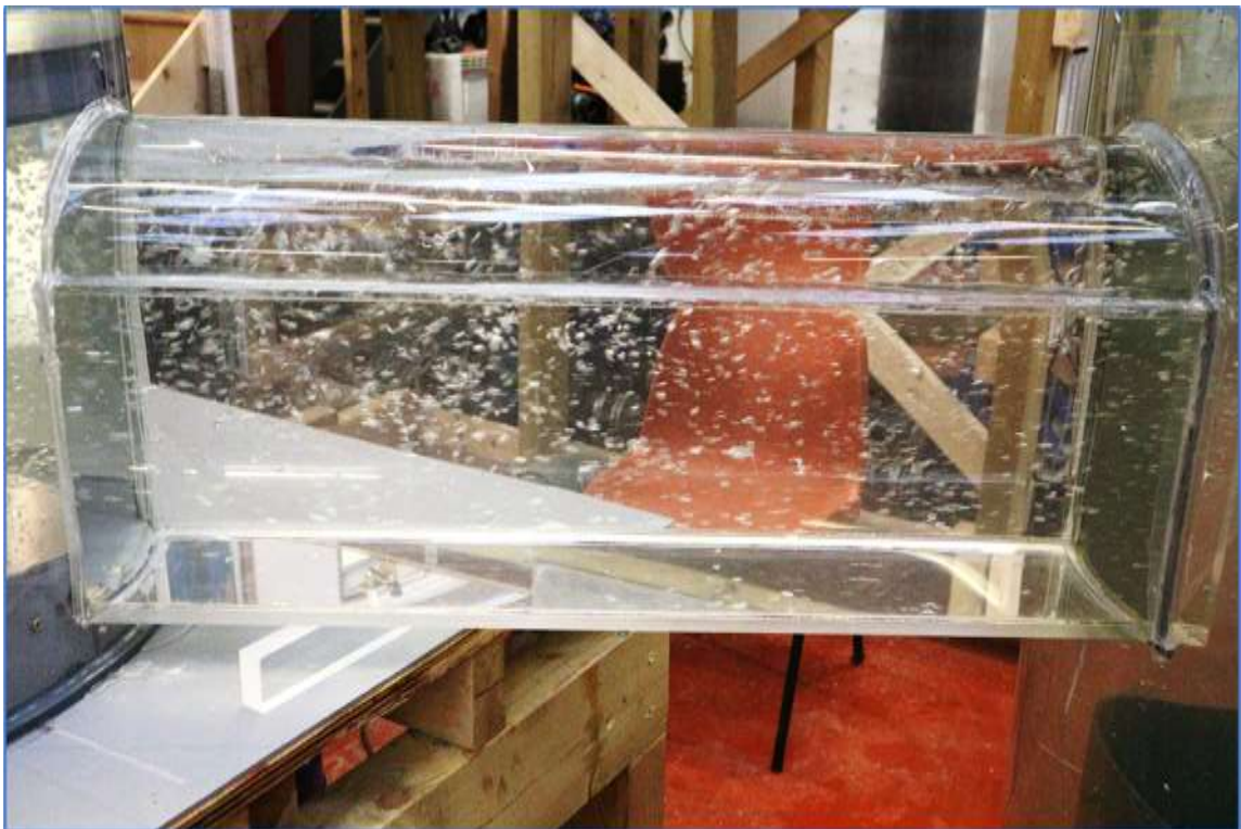
Image 4.06 – Flow conditions within the truncated outlet Culvert at 7500 l/s
