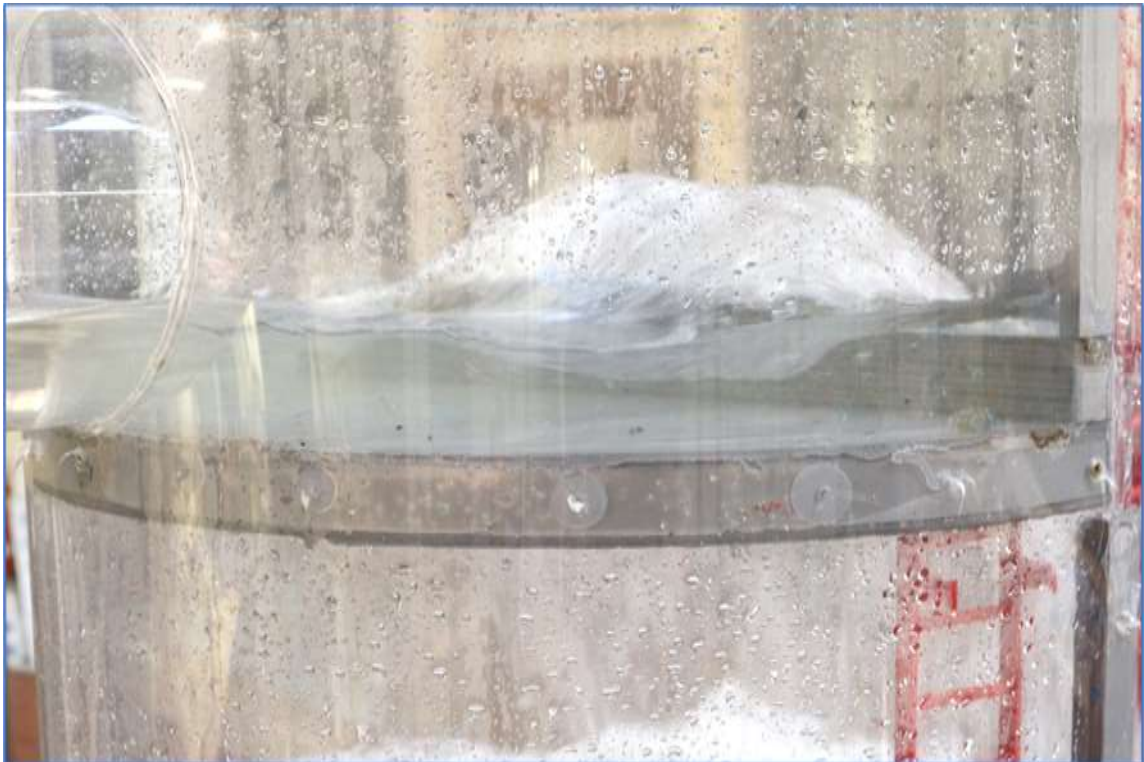
Image 4.23– Absence of settleable solids at Level 1 at a flow rate of 1400 l/s
