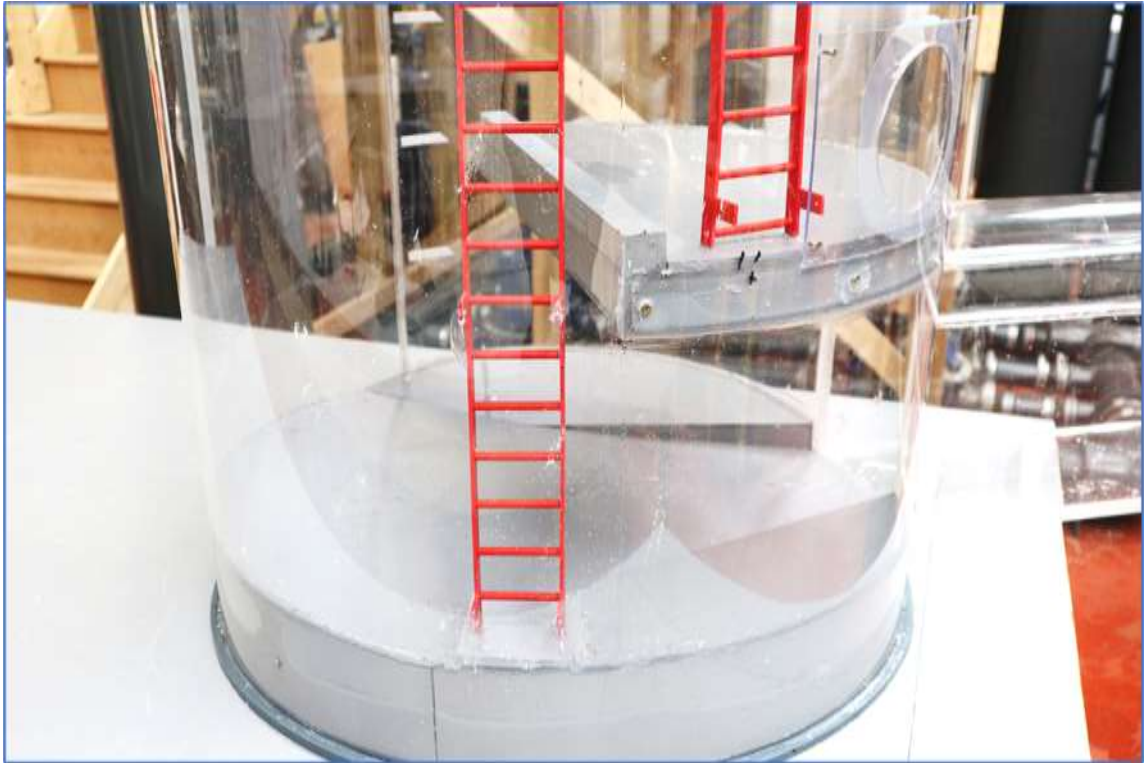
Image 1.04 – Level 4 platform and the base of the drop shaft at Level 5
