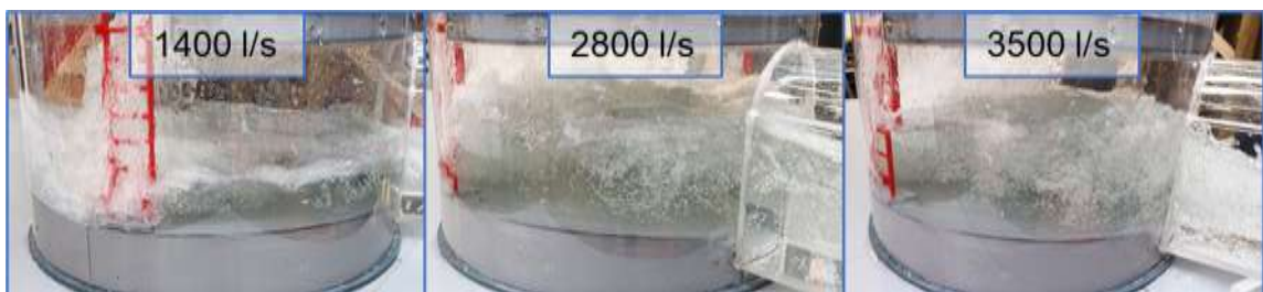
Image 4.15 – Flow conditions at Level 5 at flow rates of 1400 l/s, 2800 l/s and 3500 l/s
