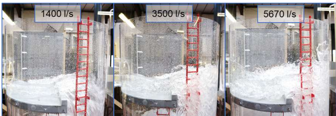
Image 2.02 – Flow conditions at Level 1 platform at a range of flow rates
