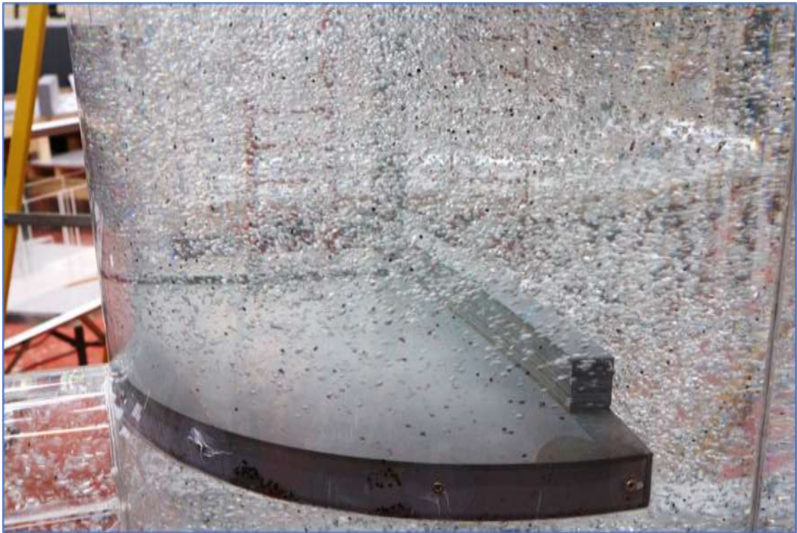
Image 4.18 – Solids in suspension at Level 4 at a flow rate of 7500 l/s
