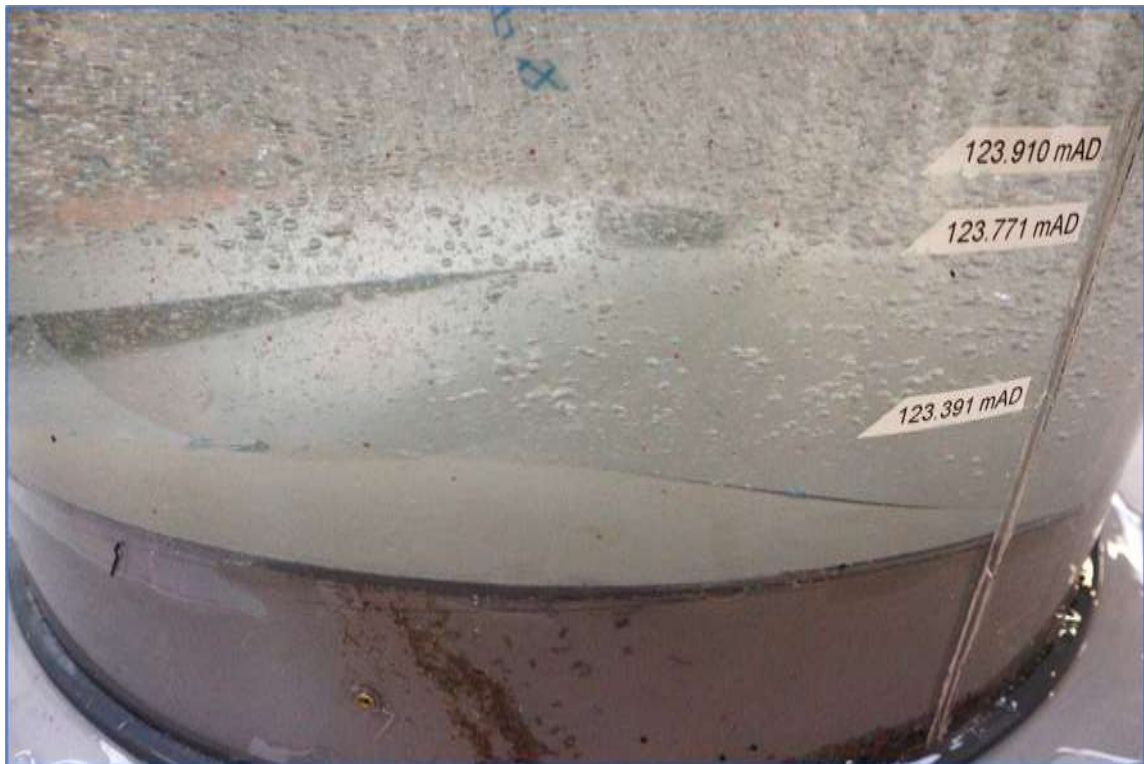
Image 4.21 – Solids suspension at Level 5 at a flow rate of 5670 l/s
