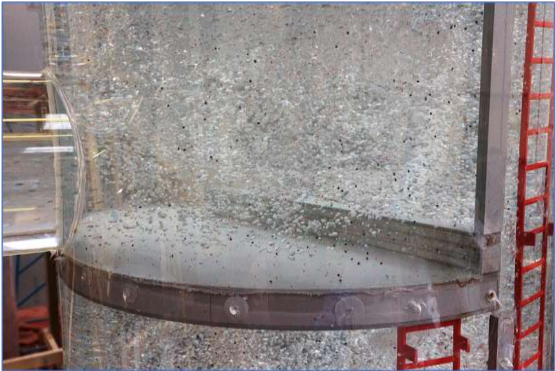
Image 4.17 – Solids in suspension at Level 1 at a flow rate of 7500 l/s
