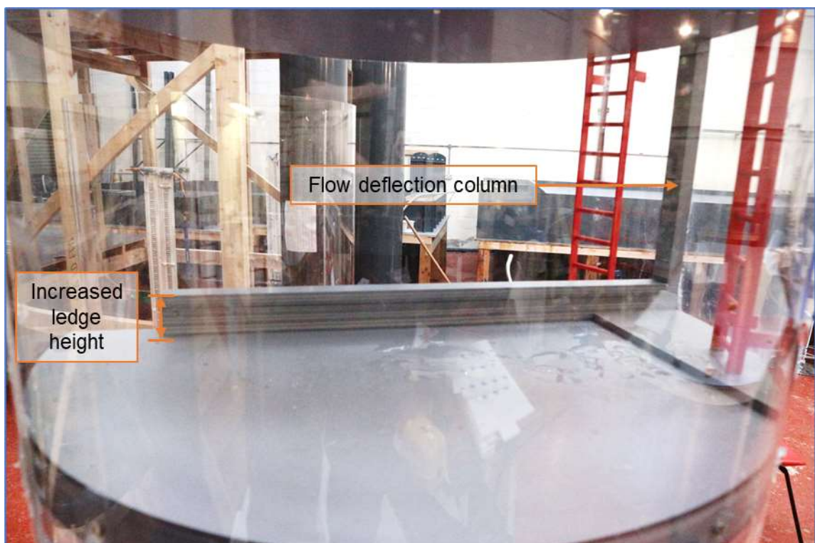
Image 3.01 – Proposed modifications installed in the physical hydraulic model
