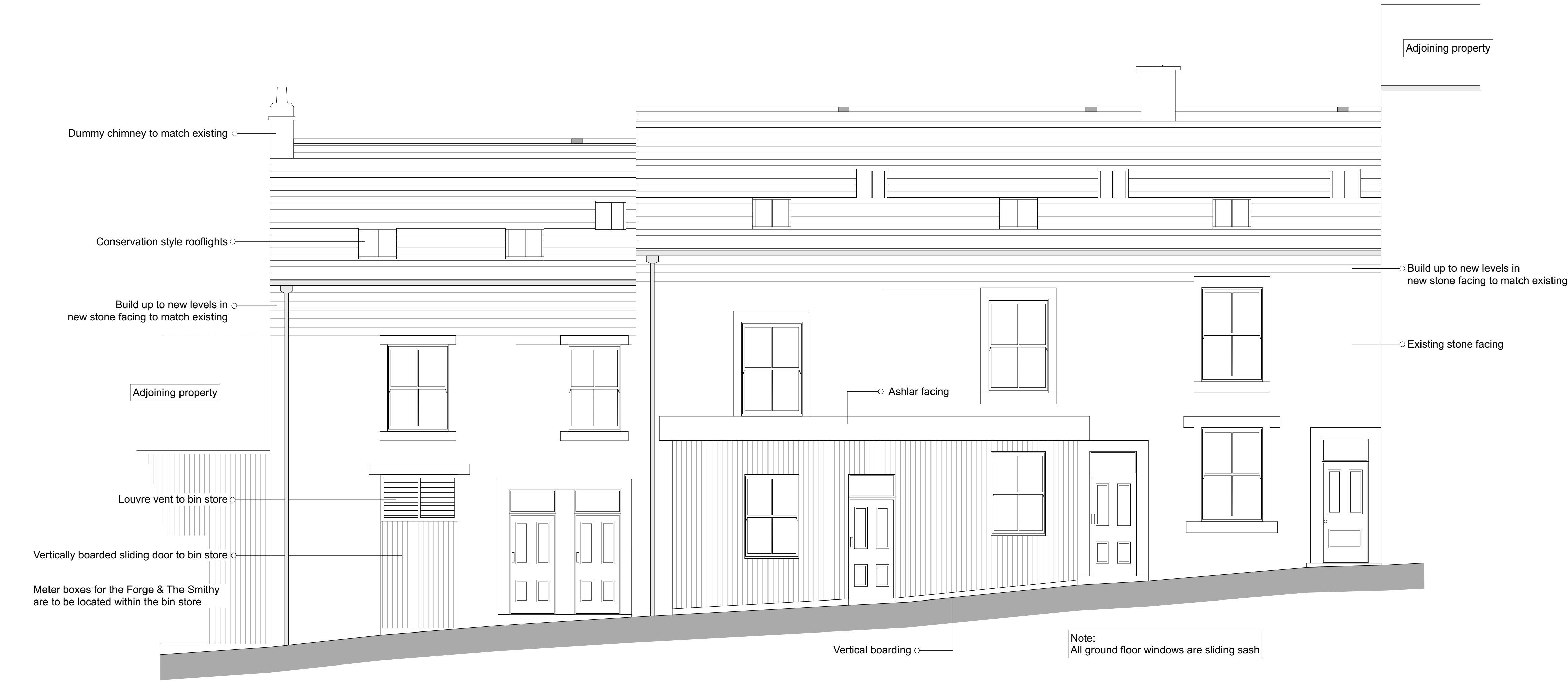
Elevation NW - Paradise St.
