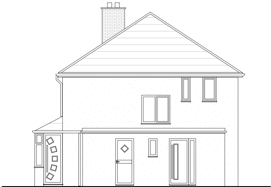
Existing North (Side) Elevation
