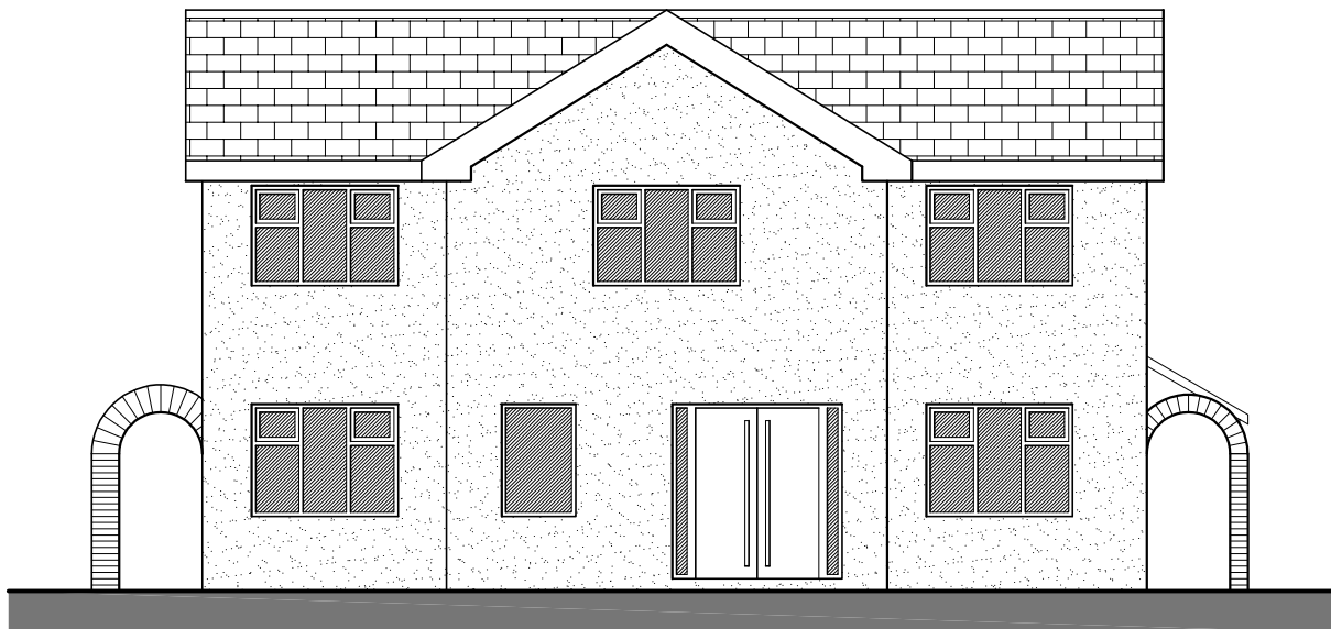
Existing Front Elevation 1:100
