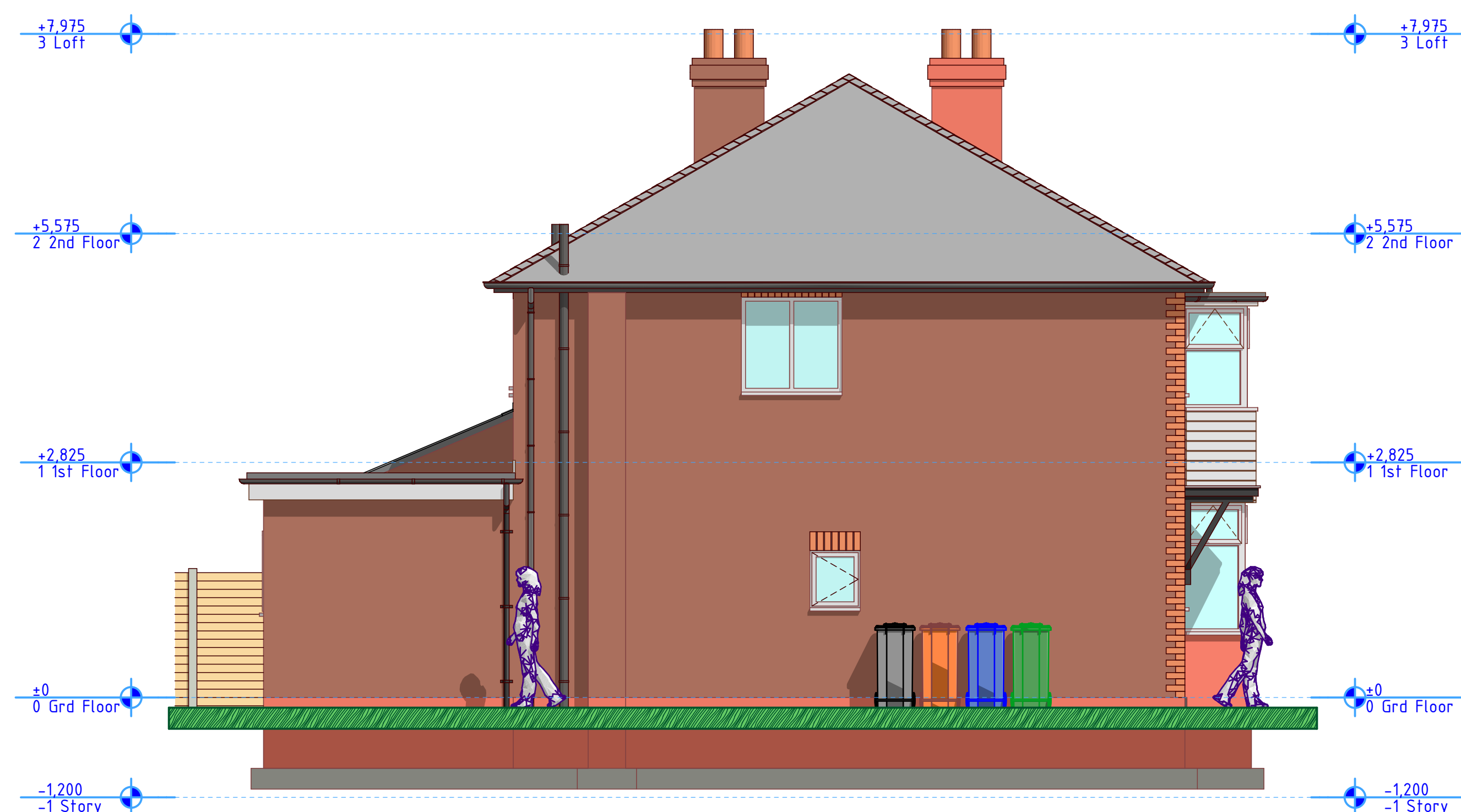
7 Existing Side Elevation 2 1:50
