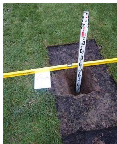
Figure 5: The gardens are finished with turf. The overall cover system depth is 600mm:
