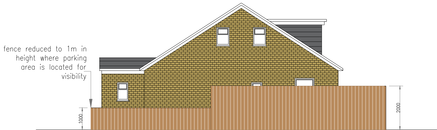
PROPOSED FENCING SIDE ELEVATION (CANUTE ST)
