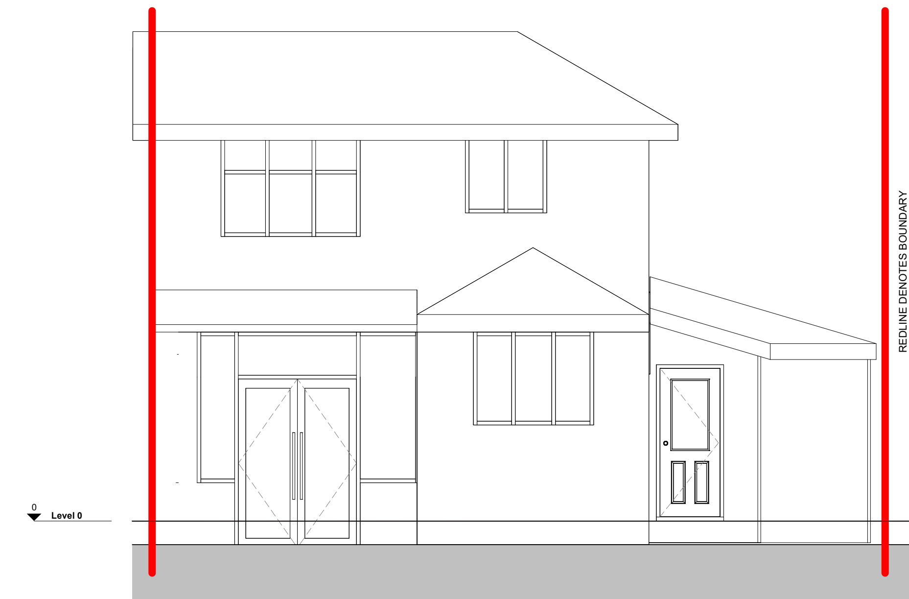
E1 EXISTING REAR ELEVATION 1 : 50
