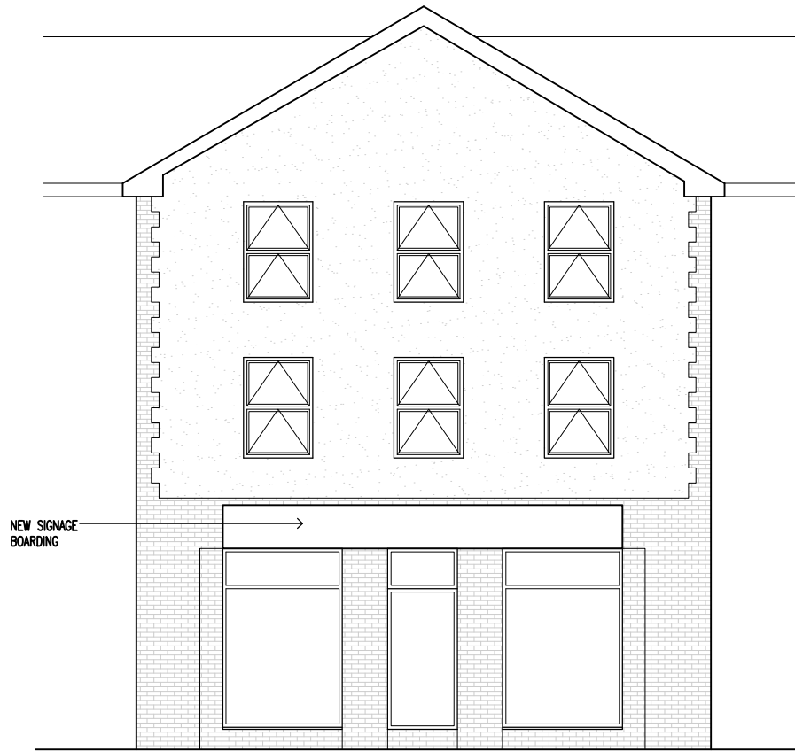
PROPOSED FRONT ELEVATION 1:100 @ A3
