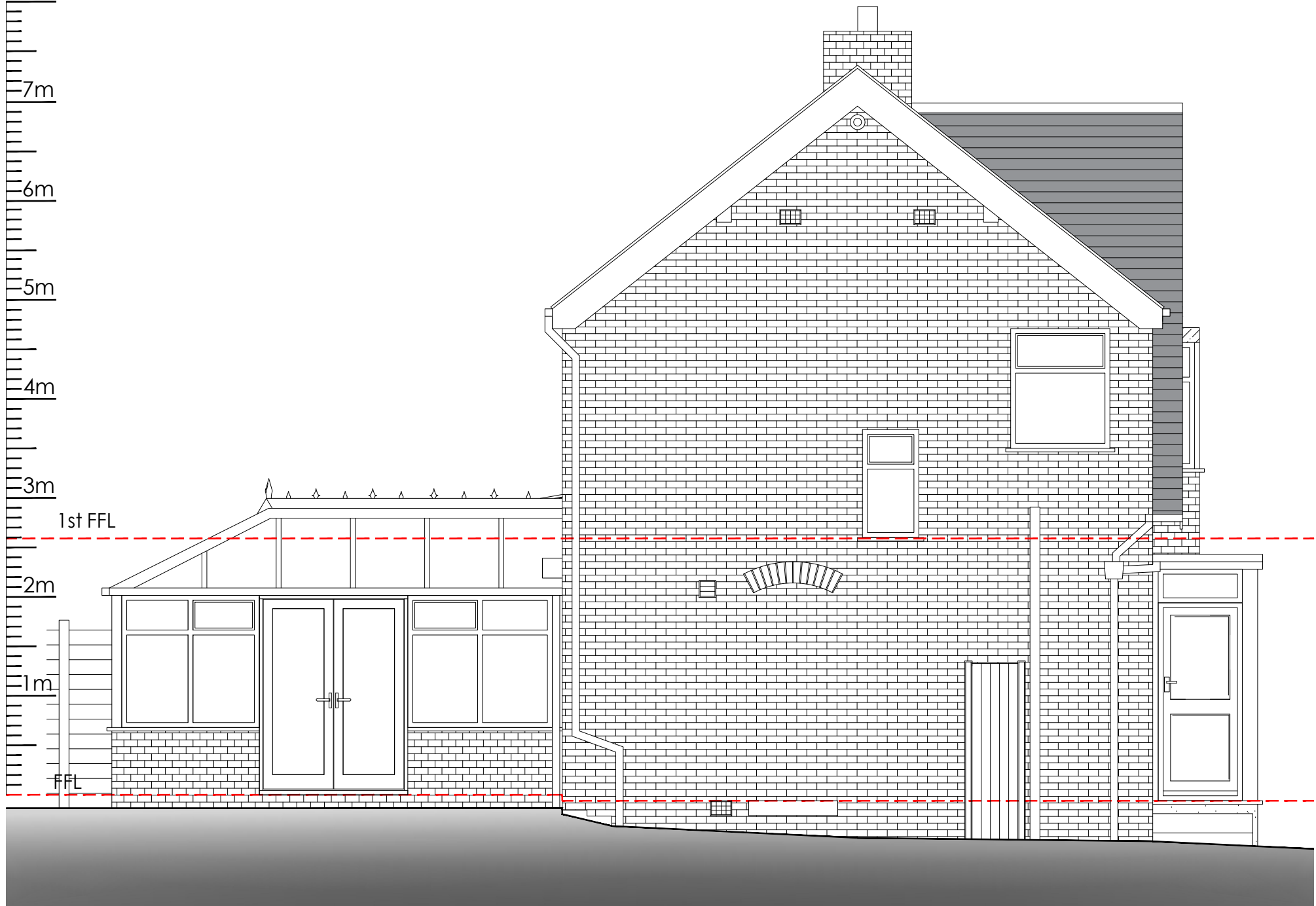
side elevation - as existing scale 1:50 @ A1
