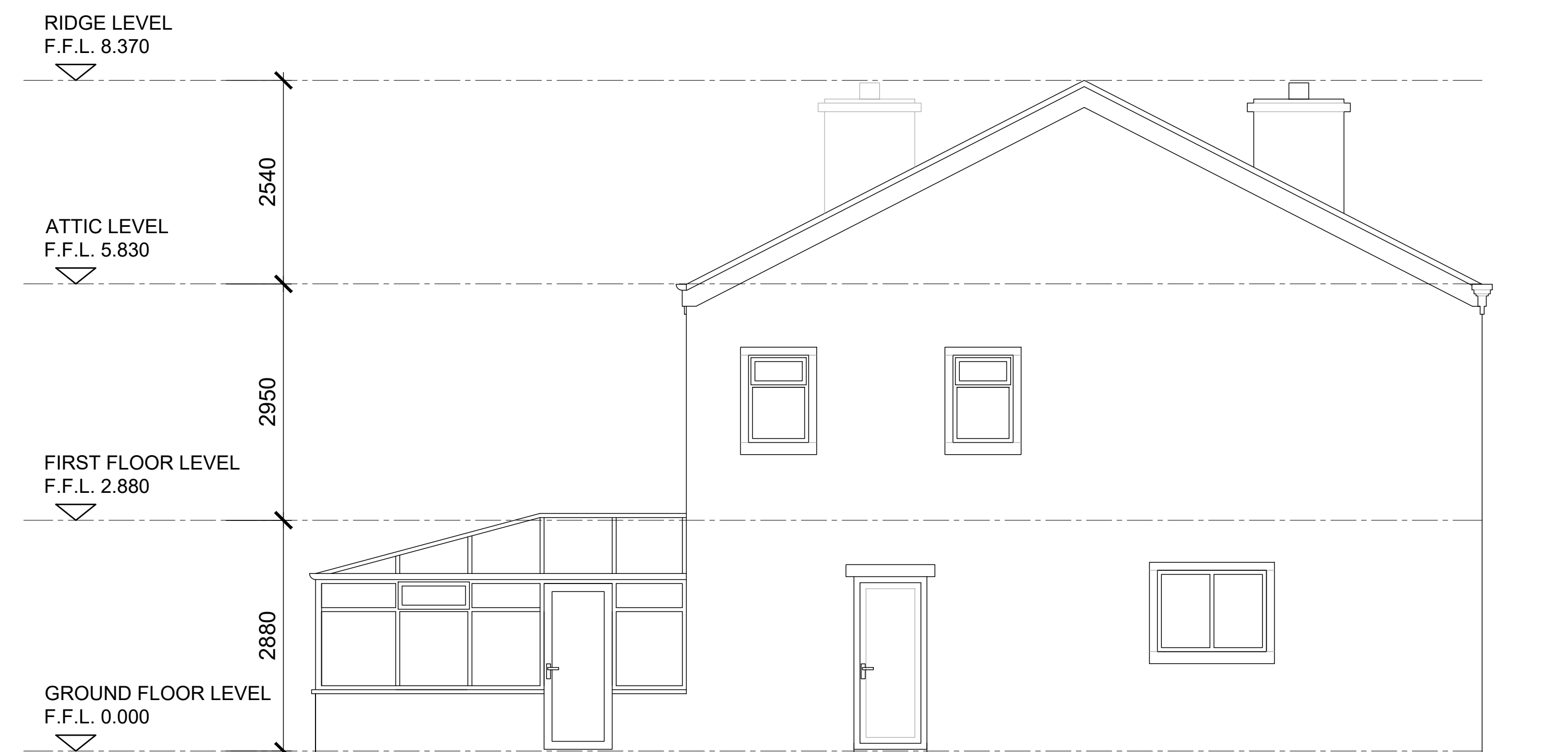
EXISTING SIDE ELEVATION
